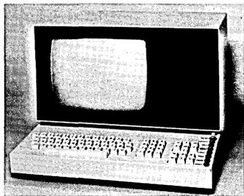
12" Green Ball Brothers monitor with enclosure measuring 19" x 16.5" x 14". Room inside to mount a Ferguson single board computer or small SS-50, S-100 system. (Power supply available, see below.) Requires +15 volts DC. @ 1.5 amps, noncomposite (separate sync) input. A sync separator schematic is available. It is also possible to mount a single 8" disk drive or two of the new slim line 8" disk drives in this enclosure. All units are used, and have been 100% tested.
