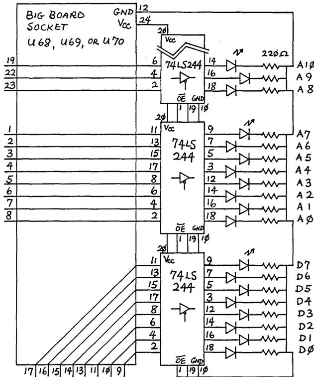
Mini Front Panel Z80 Socket Connection
