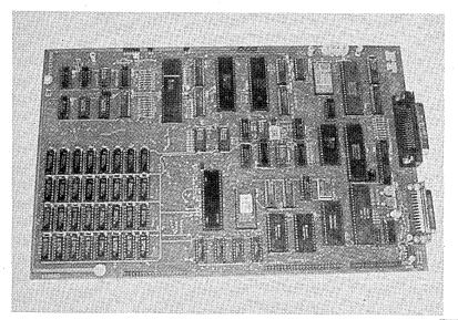
**ASSEMBLED** AND TESTED **BOARD WITH** 64K of RAM
