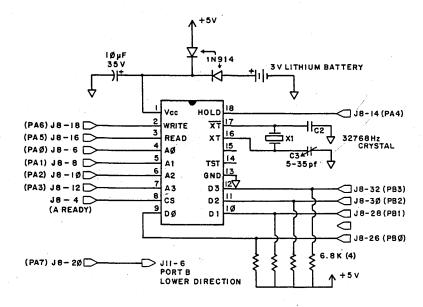
4" of wire between the IDS and the card. AFTER you have checked your wiring, cut the unused wires as close as possible to the socket. Solder the battery leads to the battery as quickly as possible to minimize battery heating.
