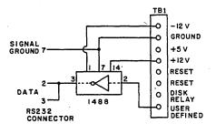
The 1488 translates the TTL signals to RS-232 levels. I have shown the data signal connected to both pins 2 and 3. This is because of an idiosyncrasy in the RS232 standard which means that your printer may expect incoming data on either pin 2 or 3.
