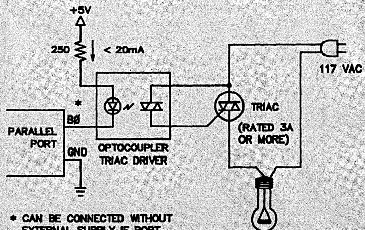
\* CAN BE CONNECTED WITHOUT EXTERNAL SUPPLY IF PORT WILL DRIVE LED (SEE TEXT).
