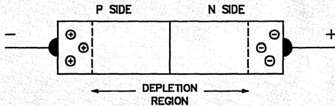
**CONNECTING P TO MINUS AND N TO PLUS CAUSES MORE COMBINATION, SO THE DEPLETION REGION GETS BIGGER. CURRENT FLOW IS BLOCKED.**
