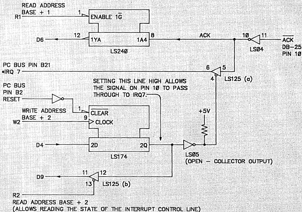
\* SINCE ALL THE PINS ON THE MICROSPHERE CARD ARE ETCHED ON THE EDGE CONNECTOR (UNLIKE SOME EXPENSIVE CARDS), IT IS POSSIBLE TO CHANGE THIS WIRE TO AN UNUSED INTERRUPT IF YOU DO IT CAREFULLY (IRQ7 IS USED BY PRINT SPOOLERS). UNUSED INTERRUPTS ARE:
