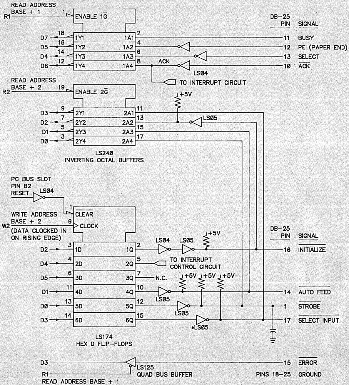
\* LS05's HAVE "OPEN COLLECTOR" OUTPUTS, MEANING WHEN THE OUTPUT IS ZERO, THEY PULL DOWN ALMOST TO GROUND, BUT WHEN IT IS ONE, THE OUTPUTS DISCONNECT THEMSELVES (ALLOWING PINS 1, 14, 16, AND 17 TO BE DRIVEN FROM THE OUTSIDE WORLD). THE "PULL-UP RESISTORS" ARE NECESSARY TO PULL THE OUTPUTS UP TO A LOGICAL ONE.
