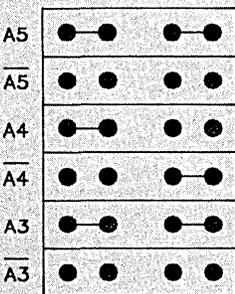
A8 TO MODIFY THE ADDRESS, CUT AND REMOVE EXISTING BOARD TRACE. SOLDER A WIRE ACROSS DESIRED PADS.
