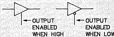
BUFFERS AND INVERTERS WITH OUTPUT ENABLE: WHEN OUTPUT IS ENABLED, SIGNAL FLOWS THROUGH AS NORMAL. WHEN NOT ENABLED, IT'S AS IF OUTPUT IS DISCONNECTED FROM CIRCUIT (THIS IS CALLED "TRI-STATE").
