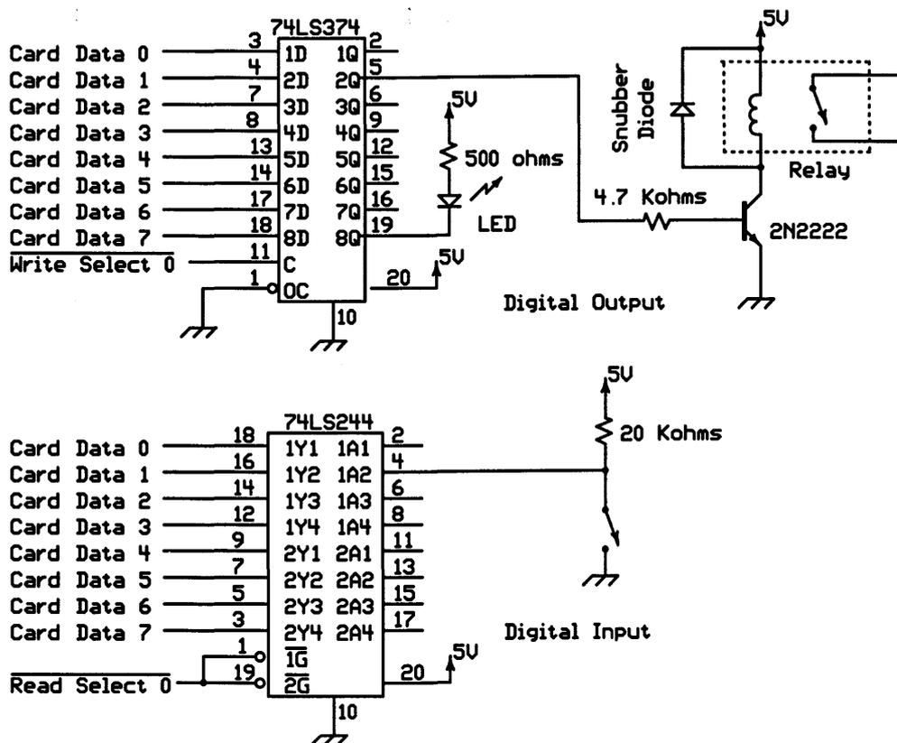
(I/O read) signal is low. When we write it, the IOW (I/O write) signal is low (memory reads and writes have their own signals). That's all there is to it — watch the I/O control lines to see if we're reading or writing (and the AEN line to make sure it isn't the DMA), and you're in business.
