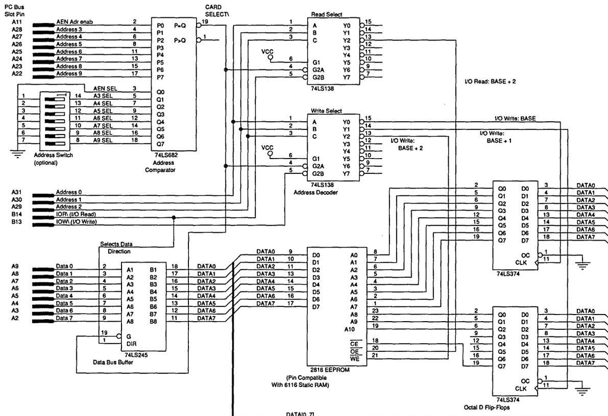
we can't dedicate any of the memory space to EEPROM so I've designed it to use the I/O space. Even then, there isn't enough free I/O space to support 2K bytes (only 10 lines, or 1 K, of I/O is brought out to the PC bus, with much of that dedicated to other purposes).
