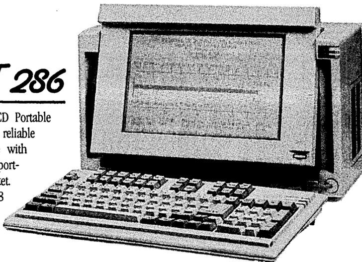
resolution 640x400 super twisted LCD with adjustable intensity and screen-angle. The screen size is 9.5"x6". It's as readable as a CRT. You can also plug in a digital or analog color monitor or a digital or composite
