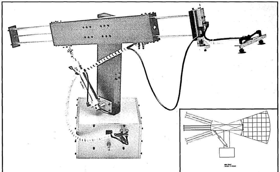
Figure 1 — BR 100 Series Pick and Place Robotic Arm.
