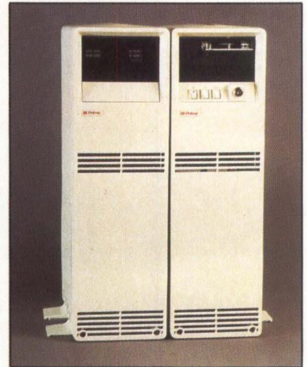
Based on the Intel 80386 micro-processor, the Prime EXL 316 is the first multiuser system to transparently run commercially available UNIX and MS-DOS programs. A fully configured system offers 8M bytes of memory and more than 1G byte of disk storage.
