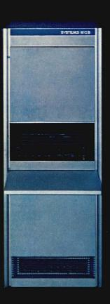
SYSTEMS 810B Word length—16-bit Cycle time—750 nanosec. Maximum core memory—32 MODERN DATA/November 1970
