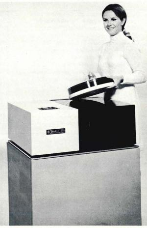
Fig. 1. The Talcott 9311, a plug-to-plug compatible 2311 diskpack drive, available from Talcott Computer Leasing and manufactured by Singer-Friden.
