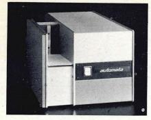
The Automata 3600 reads intermixed stacks of variable length cards at speeds up to 300 cpm. This includes pre-punched, pre-printed and pencil marked information on the same card.
