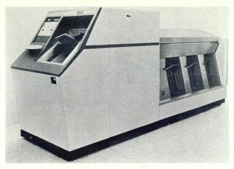
The Input 80 page reader, an OCR reader produced by Recognition Equipment capable of reading machine-printed or handprinted input at speeds of 3,600 characters per second.
