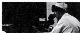
Select resistor chip, adjust to exact value, coat with silicone and encapsulate.
