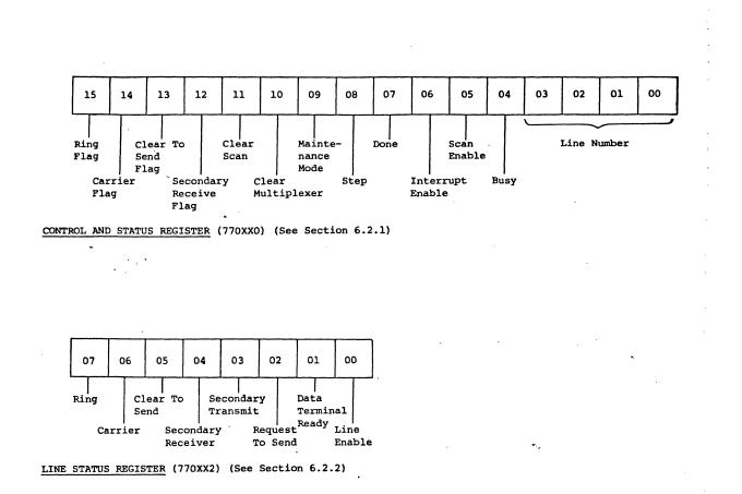
Figure 6-4: Modem Register Formats
