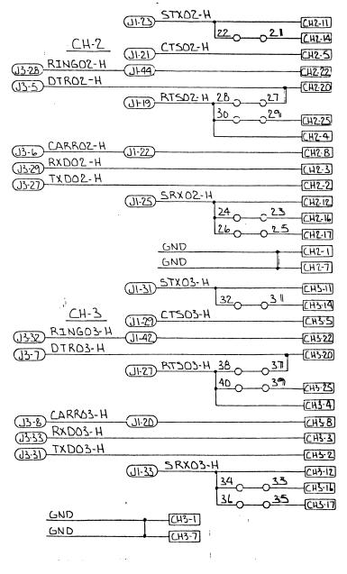
Figure 5-3: Wiring Chart For Modem Connection
