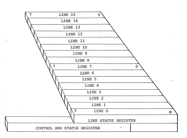
Figure 6-3: Modem Registers
