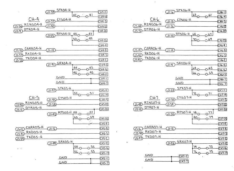
Figure 5-3: Wiring Chart For Modem Connection (Con't.)
