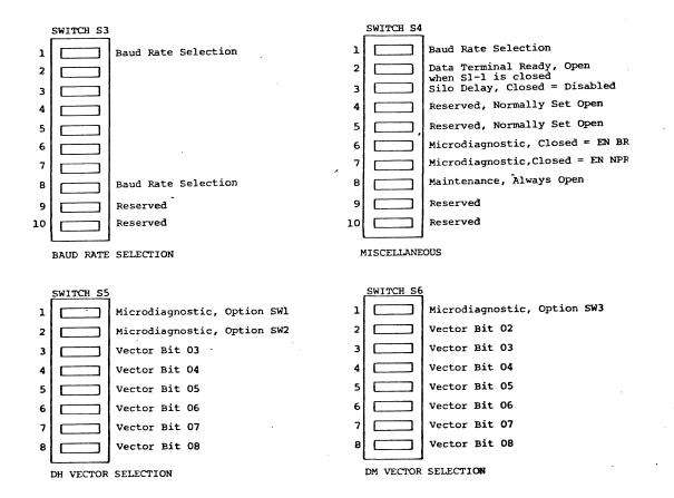
Figure 3-3: DH/DM Switch Descriptions
