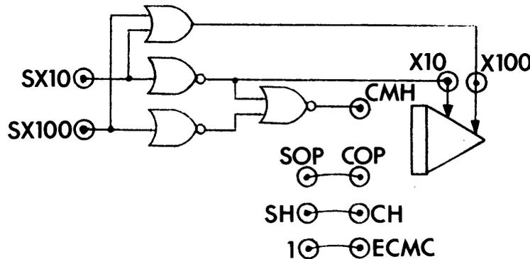
The patching to CMH, COP, and CH provides a Master Hold in case X1000 is inadvertently requested by the operator. This is optional, but highly recommended.
