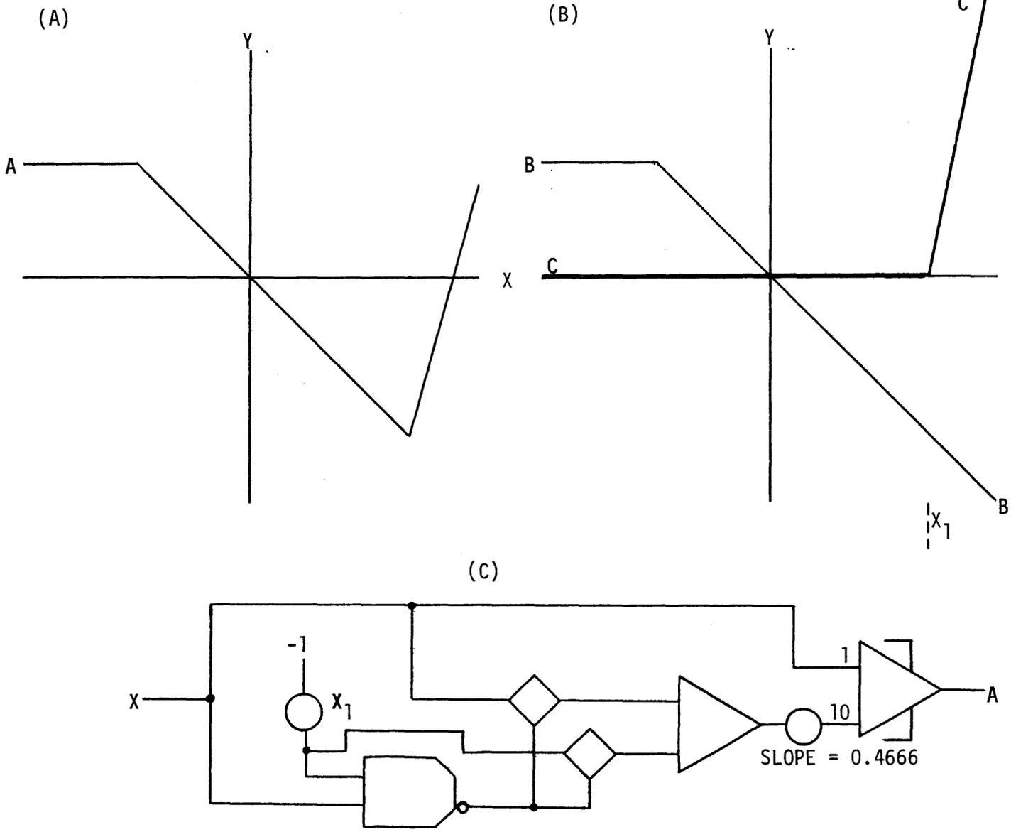
Figure 5-14 Example of an Arbitrary Characteristic
