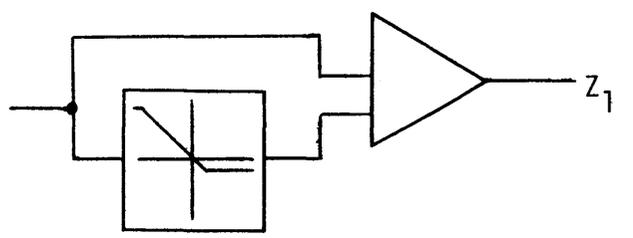
Figure 5-13 Horizontal Shift of a Characteristic
