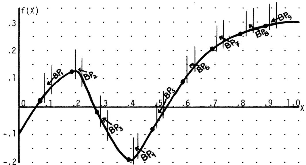
Figure 3.6 Function to be Programmed by the E3.17 VDFG
