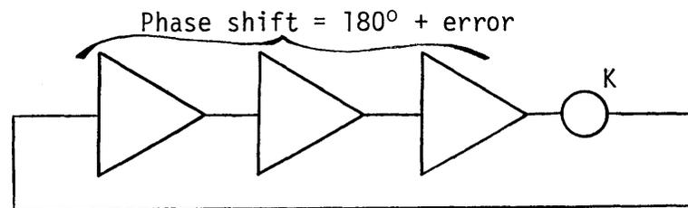
Figure 5-5 Algebraic Loop with Odd Number of Summers
