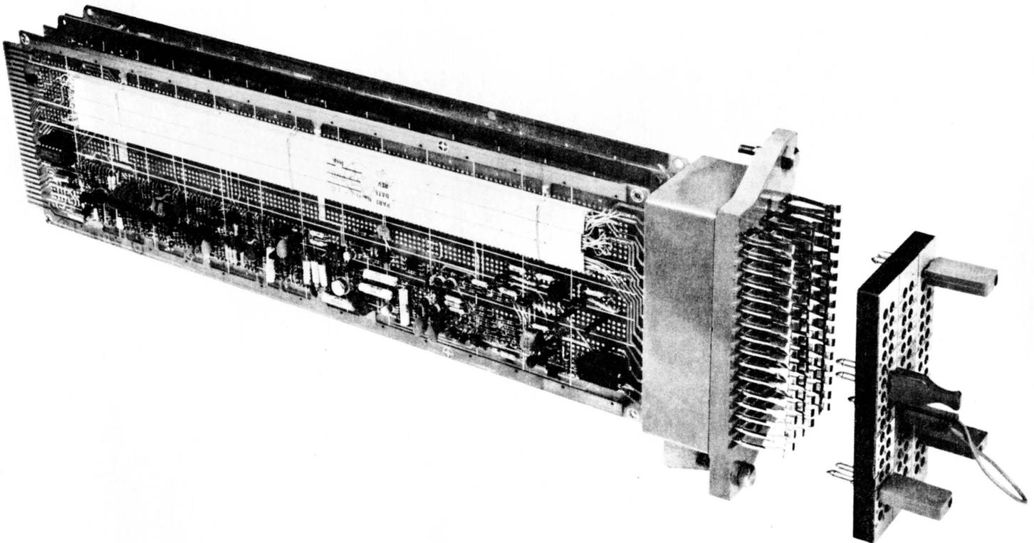
Figure 1-4 Patchboard Module, Patchbay Pin Block, and Circuit Cards
