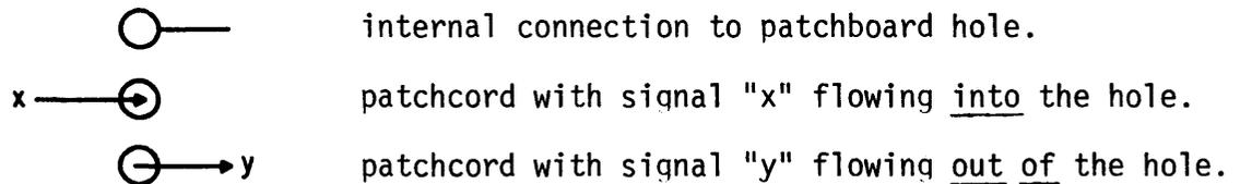
The concept of signal flow direction should not be confused with voltage or current polarities. Signals flow from sources to destinations without regard to polarity or logical state.
