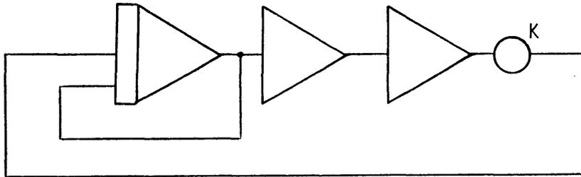
The feedback resistor for the integrator must be the same resistor as in the summer which it replaces.
