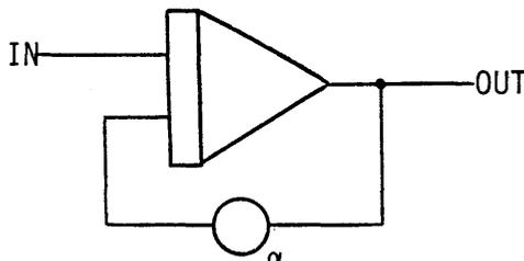
The corner frequency (6db/octave roll off point) is  $\alpha$  radians/second.
