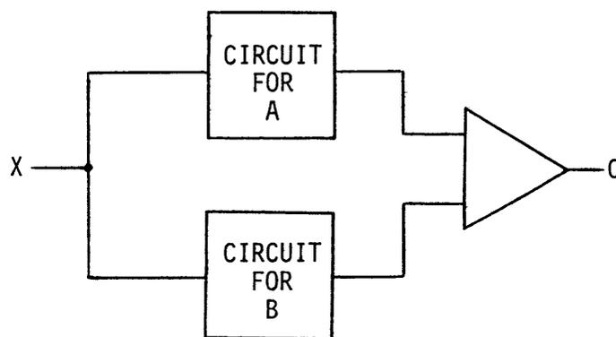
Figure 5-11 Sum of Two Transfer Characteristics
