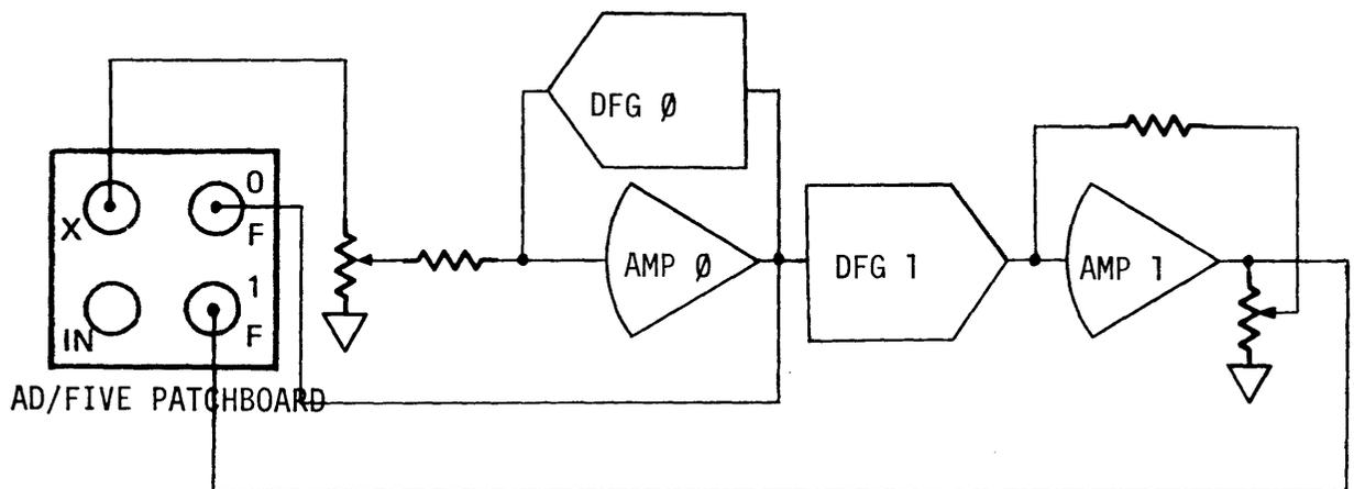
Figure 1.2 DFG Variable Breakpoint Configuration
