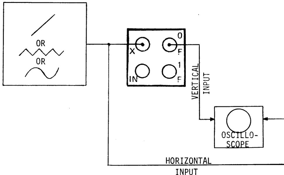
Figure 3.0 Oscilloscope Connections
