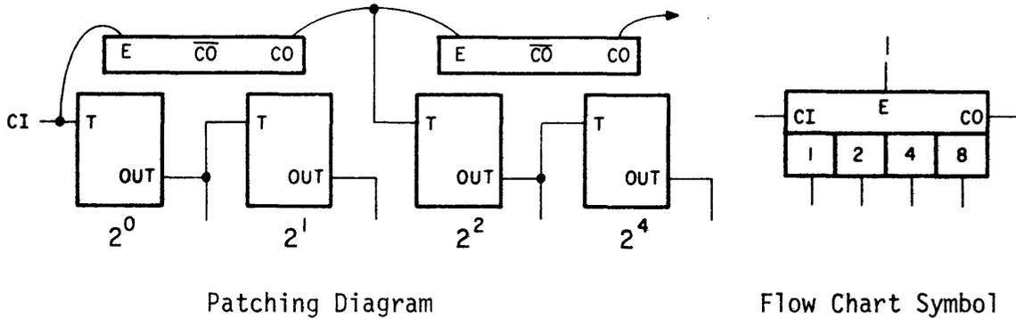
CI must be patched to the low numbered (0 or 3) flip-flop of each pair.
