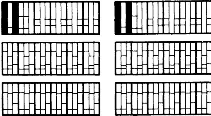
The D5.140 contains mode and time scale controls for the integrators as well as control for the electronic switches in three areas or one fourth of the AD/FIVE. When expansion Integrators/Summers are used, each set of integrator controls acts on both Integrator/Summers in a given area and row. (See D1.35 Integrator/Summer.)
