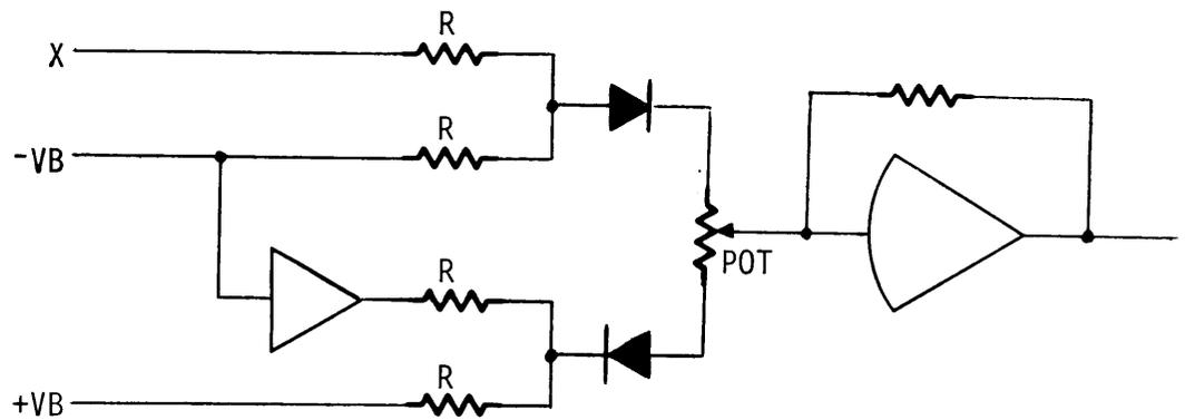
Figure 2.1 Simplified Slope Segment Circuit
