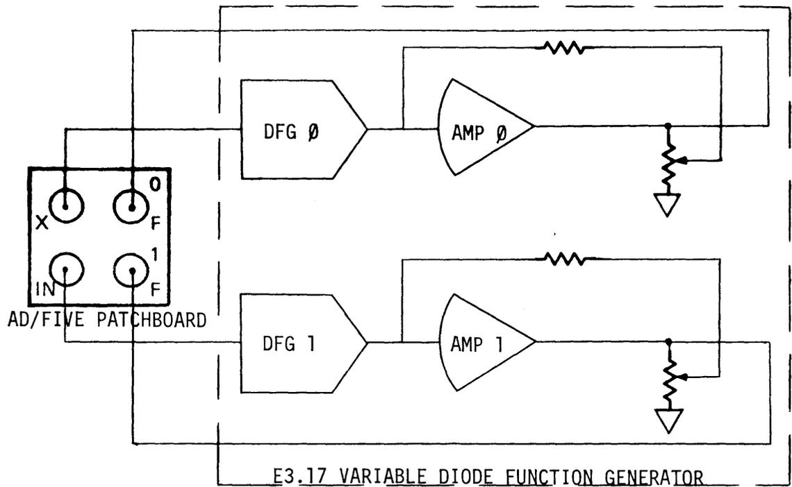
Figure 1.1 DFG Fixed Breakpoint Configuration
