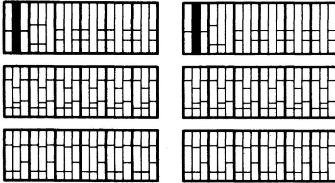
The D5.166 contains logic terminals for twelve comparators in one AD/FIVE field. The four additional comparators (beyond the normal eight) replace track/store networks, and are always enabled.
