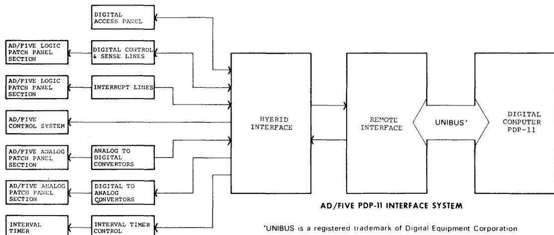
Figure 1-2 The AD/FIVE-PDP 11 SYSTEM 511
