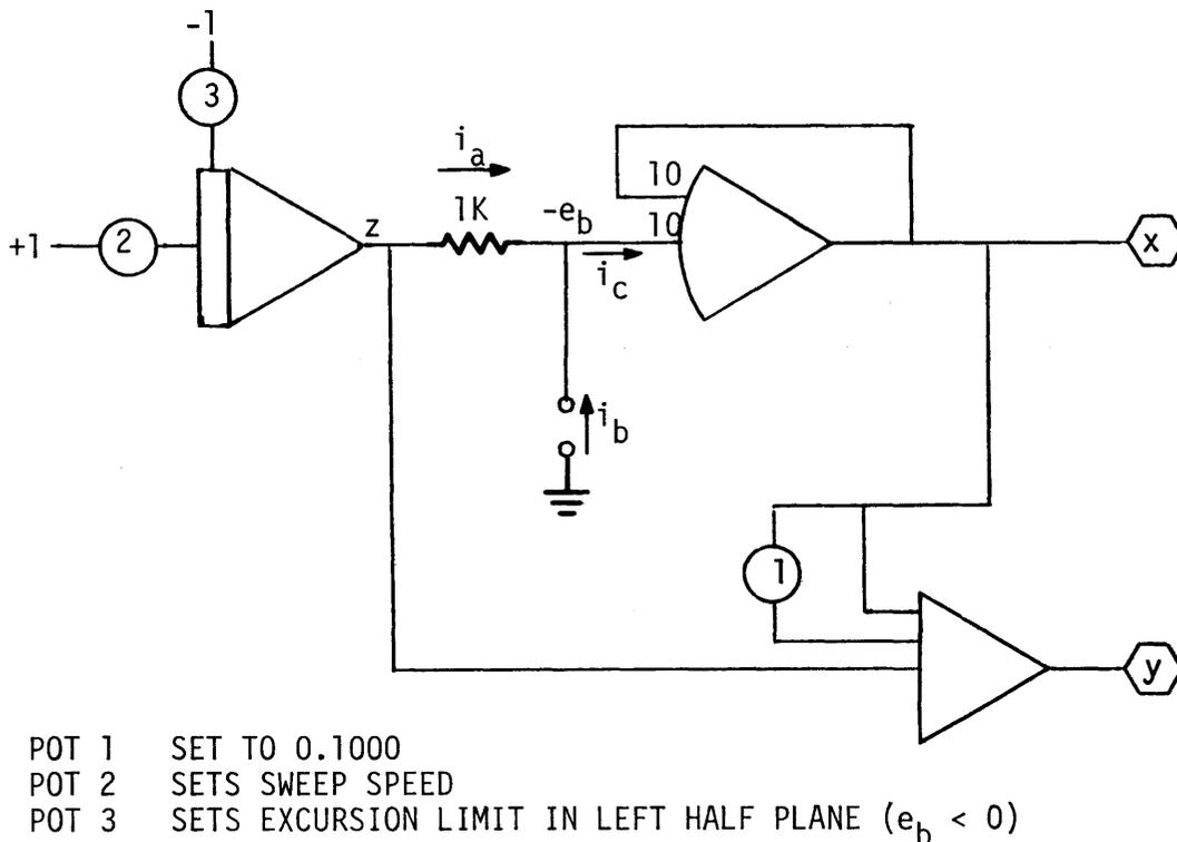
Figure 5-16 Part A Volt-Ampere Characteristic Plotter Circuit
