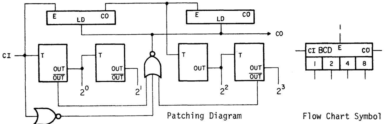
Figure 5-31 BCD Counter With Outputs
