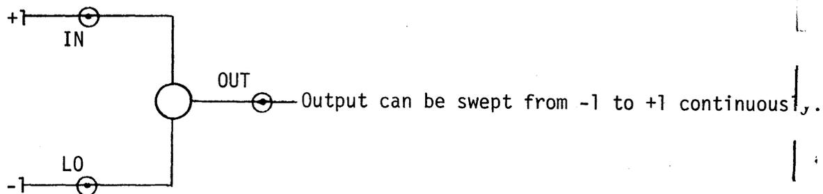
Figure 5-23 Reference Potentiometer
