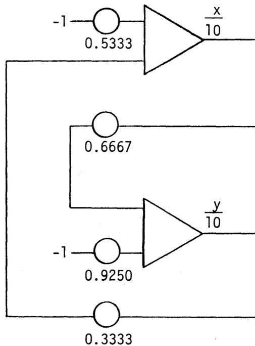
Figure 5-10 Example of Algebraic Solution
