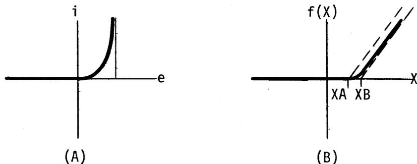
Figure 2.3 Actual Diode Switch Characteristics
