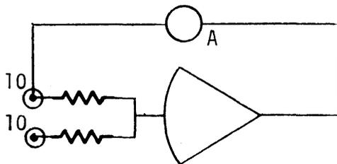
If the output of a high gain amplifier is patched to the input of a pot, and the output of the pot is patched to an input labelled 10 on the patchboard, then the gain of the remaining 10 input will be:
