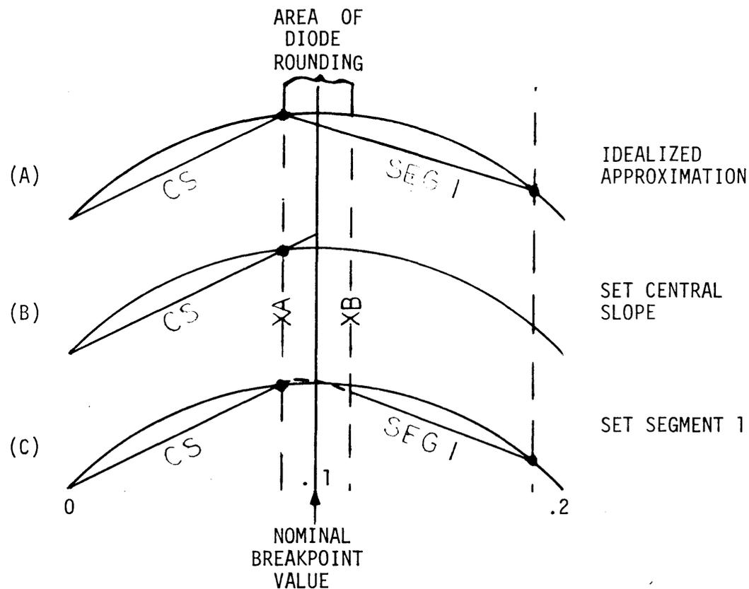
Figure 3.3 Diode Rounding: Setting  $f(X)$  Before Nominal Breakpoint
