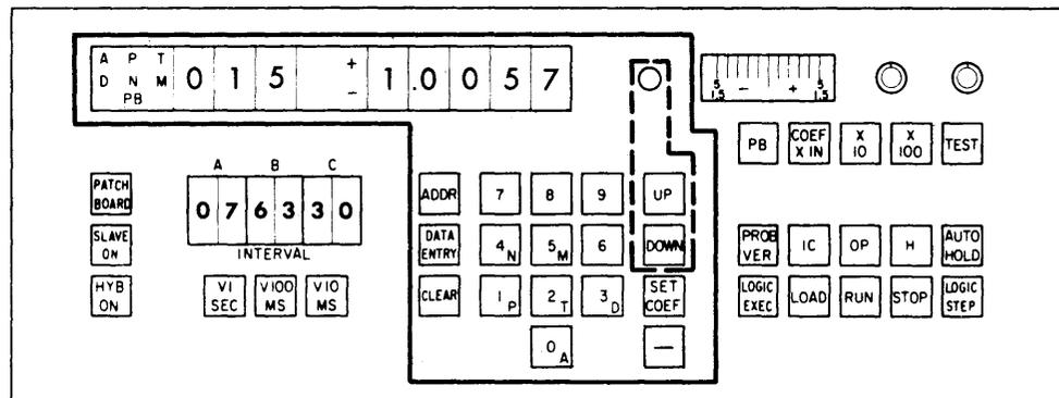
Coefficient Setting System Displays and Controls
