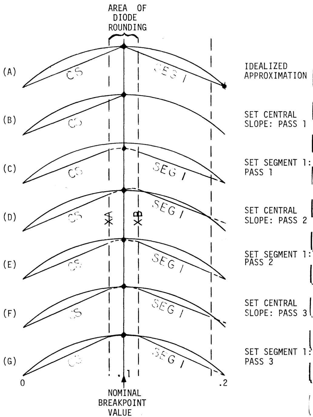
Figure 3.2 Diode Rounding: Setting  $f(x)$  at Nominal Breakpoint
