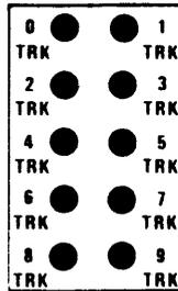
CAUTION: Addressable trunks 0 to 4 exhibit a ground connection when the AD/FIVE power switch is turned off.
