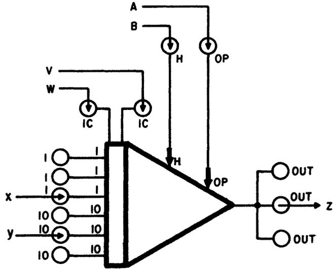
When individual integrator mode control is patched, then the mode is determined by the inputs to A and B. It will often be necessary to patch A or B to a logic zero in order to override console control of the integrator. It cannot be assumed that if A or B are unpatched that they will behave as if patched to logic zero. If A is patched to a logic one, for example, but console mode is Hold, then the integrator will not operate until B is patched to a logic zero.
