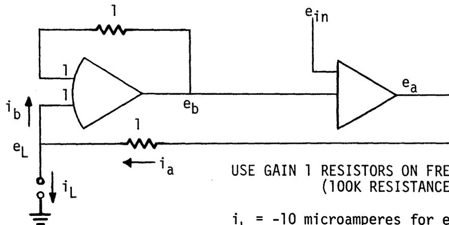
USE GAIN 1 RESISTORS ON FREE NETWORK CARD
