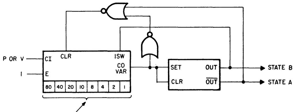
Patch the total cycle time ("A" period plus "B" period). Set the A period on the VCO counter thumbwheel switch.
