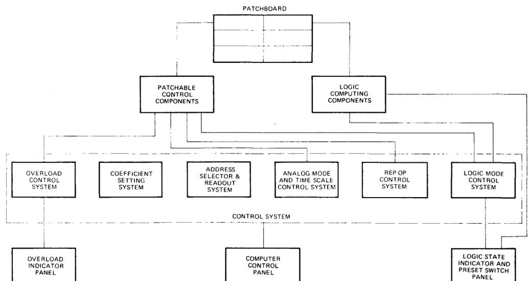
Functional Diagram for Logic and Patchable Control Components
