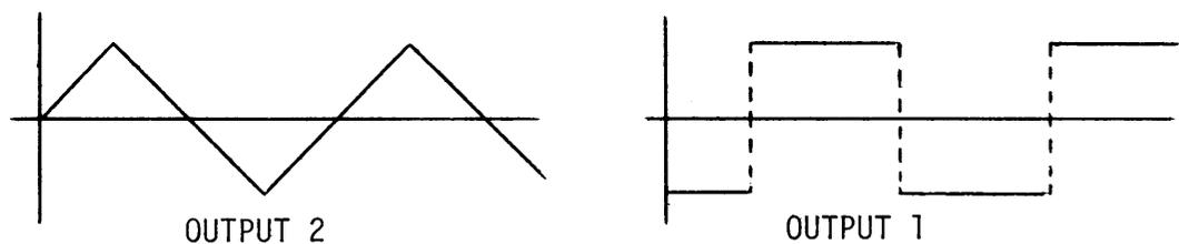
Figure 5-1 Triangle Wave Generator
