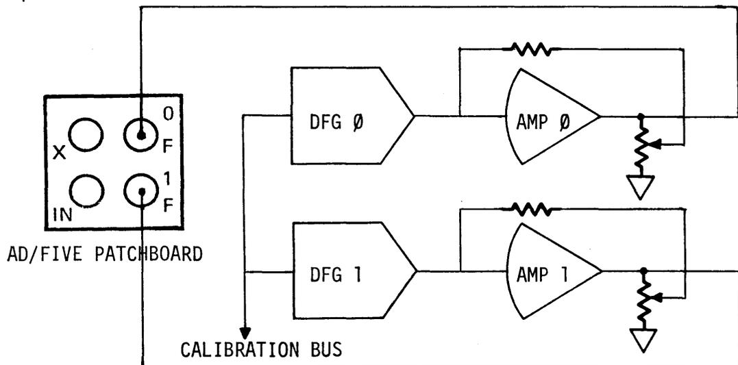
Figure 1.4 DFG Function Calibration Configuration
