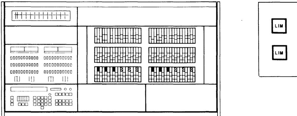
Note; X is defined as the normal value of the problem variable input to the limited amplifier as held between the limits of  $\epsilon$  and  $\rho$ . Both the upper and lower limit terminations +L and -L must be patched in order for the Limiter to be operational. The following conditions must also be observed:
