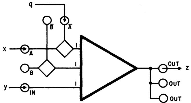
$$Z = -(Y + X) \text{ if } q \text{ is logic zero (or unpatched)}$$
