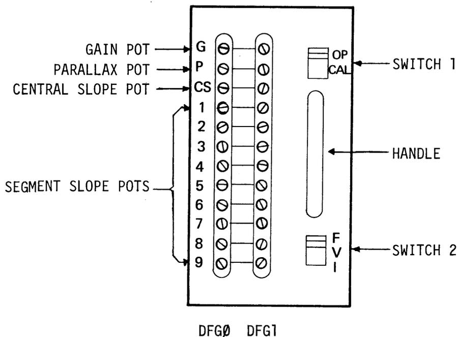
Figure 1.0 E3.17 Variable Diode Function Generator Front Panel
