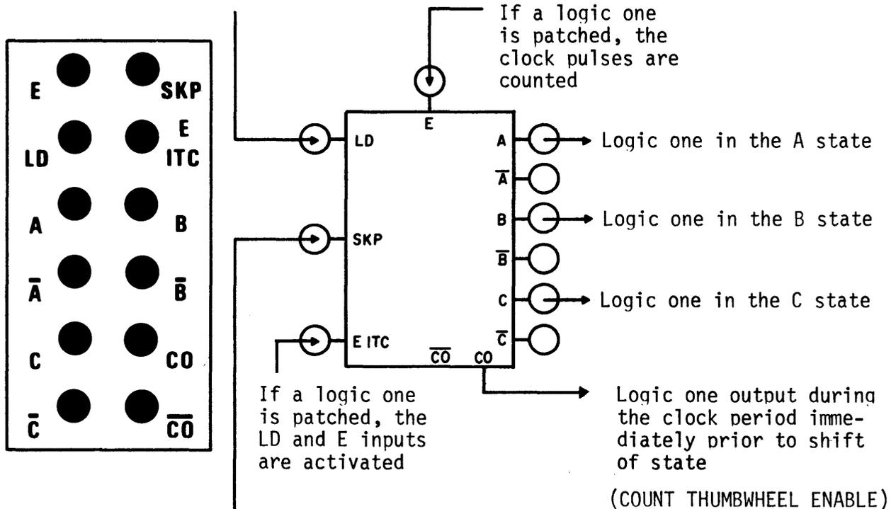
The SKP input is always active, whether or not E is a logic one. A logic one patched into SKP cancels the present state of the interval timer and advances the timer to the next state at the next enabled clock pulse. If the count has been reached and the state is ready to change when SKP goes to a logic one, then the entire next state is skipped at the next enabled clock pulse.
