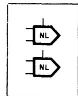
CAUTION:  $|\alpha| + |\beta| \leq 2$  must be observed when patching the multiply configuration.
