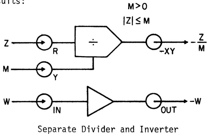
Care must be taken to avoid values of Z and M too near zero, as inaccurate results will be obtained due to inherent sensitivity of the circuit to noise for very small input signals.
