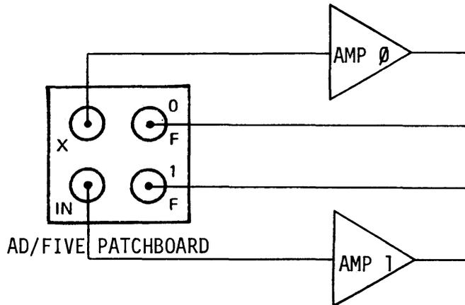
Figure 1.3 DFG Inverter Configuration
