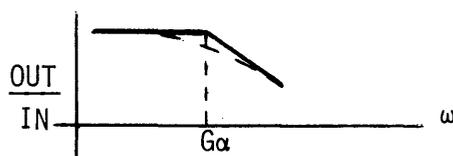
Figure 5-3 The Low Pass Filter
