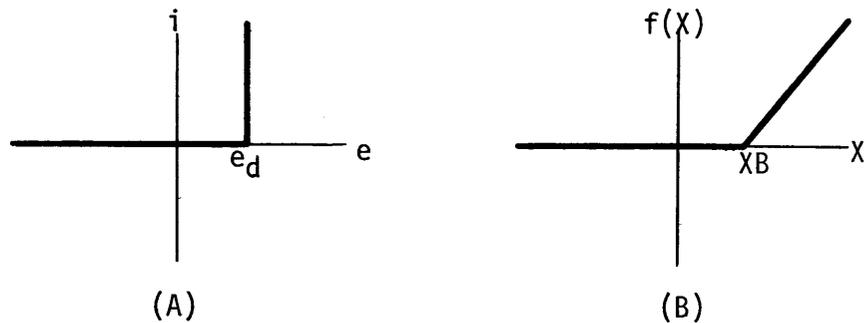
Figure 2.2 Ideal Diode Switch Characteristics
