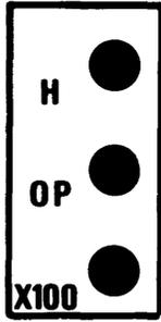
To lock an individual integrator at gain one so that it will be independent of console gain controls, patch X100 to a logic zero, and X10 to a logic zero or plus reference
