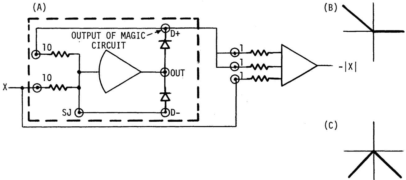
Figure 5-15 Magic Circuit and Absolute Value Circuit
