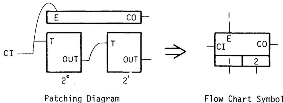
Use the CO terminal for output to another counter. The two flip-flops have a common enable. The count is incremented each time CI is logic one and there is a clock pulse. CI must be patched to the low numbered (0 or 3) flip-flop of the pair.
