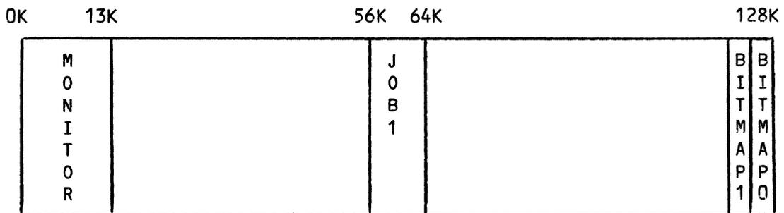
Allocation for the monitor then grows as the commands in the system initialization command file are processed. When the system encounters a SYSTEM command without an argument, the size and boundary of the monitor are finalized. At this point, JOB1 is moved to the 8KB segment contiguous with the monitor area, as shown in the diagram on the next page.
