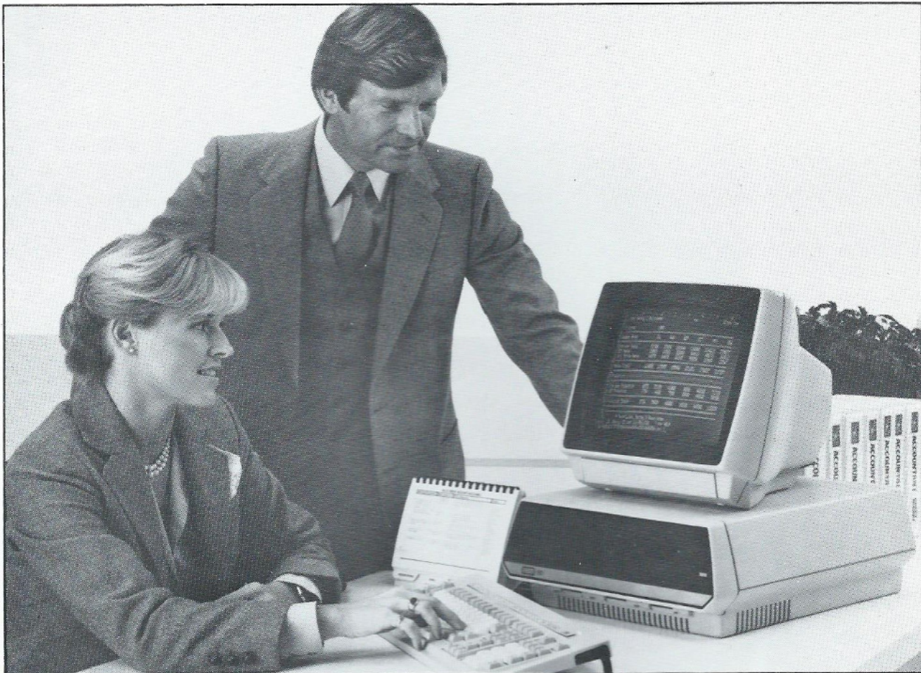
The Altos 586 microcomputer is a multi-user 16-bit system with local networking capability, communications features, high processing capacity, and wide software compatibility.
