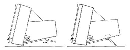
If the foot does not extend when the terminal is tilted forward, turn the screw counterclockwise to loosen it.
