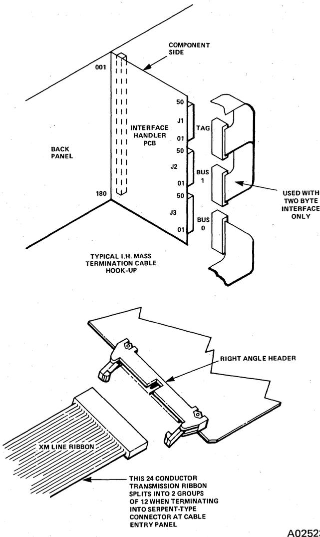
Figure 7. Transmission-Line Ribbon Cable from the Channel Interface Handler to the Cable Entry Panel
