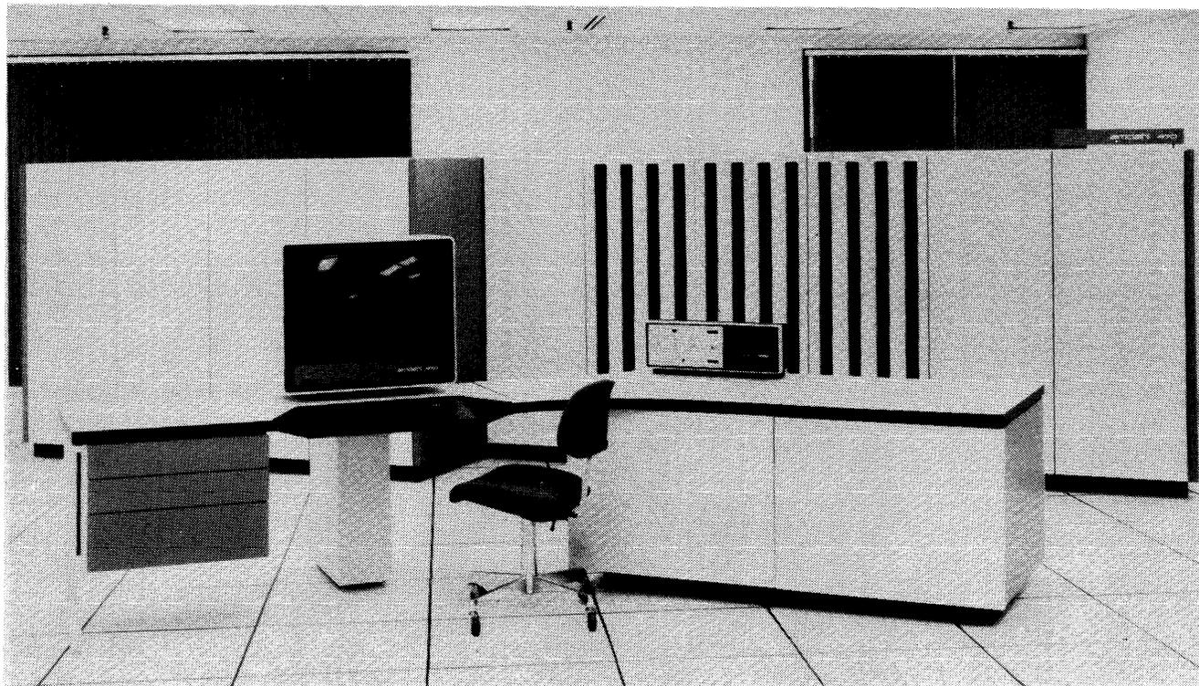
The 470V/6 System Console (foreground) features a Data General Nova 1200 minicomputer that acts as a console processor, as well as a CRT display, keyboard, and control panel. Though its rated
