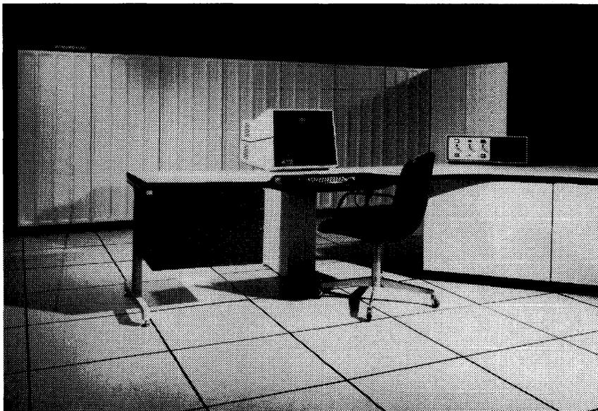
The Amdahl 470V/8, shown here, is the most powerful member in the 470 Series, with an execution rate of about 6.4 to 7.0 MIPS (million instructions per second). All 470 systems are air-cooled, and can execute any IBM System/370 software as well as utilize System/370-compatible peripheral devices.
