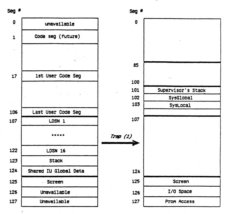
Hardware Segmentation: 24 bit address - 7 bit seg# and 17 bit offset
