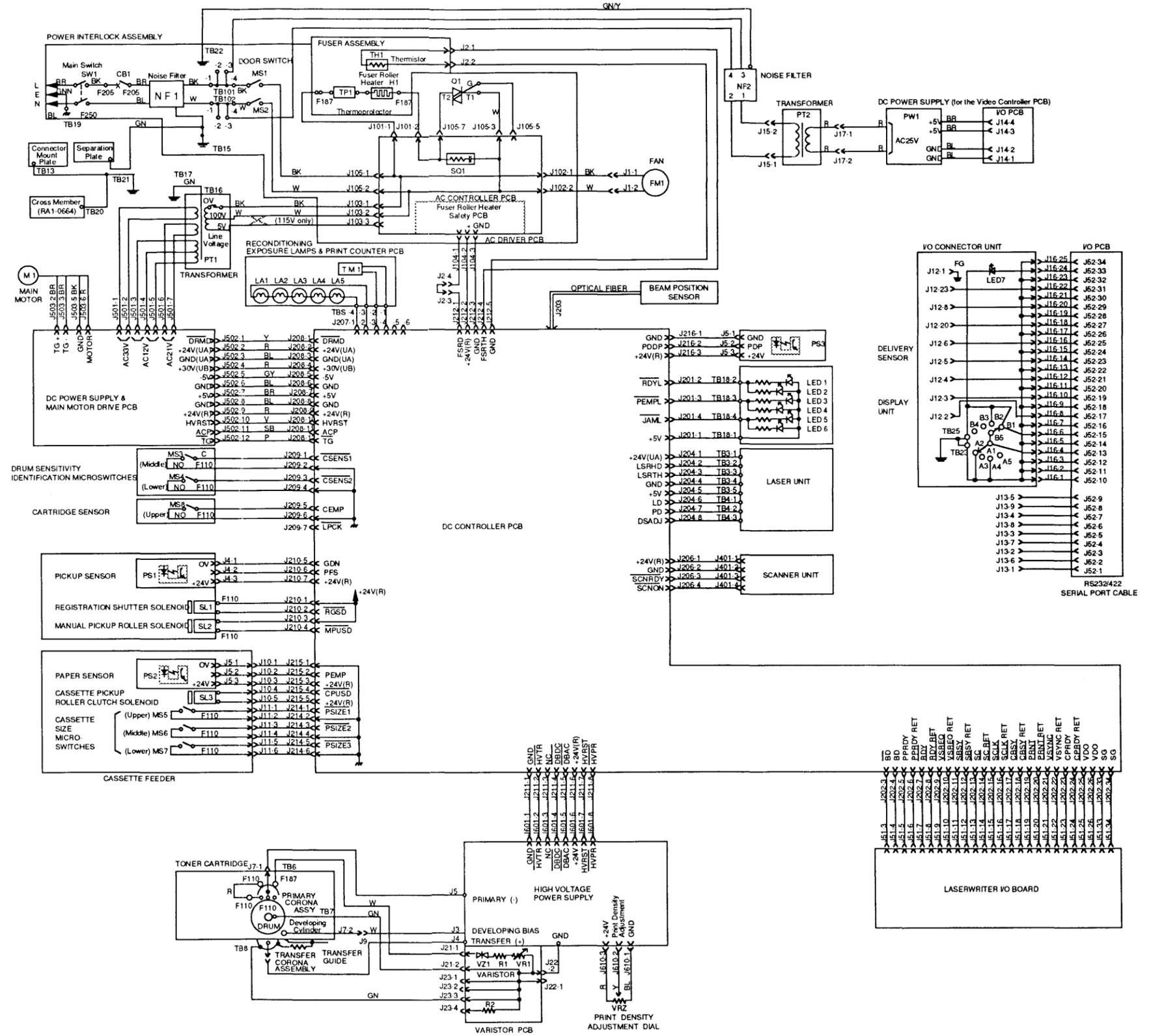
□ LASERWRITER WIRING DIAGRAM – 220V
