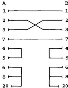
This null modem will always work since no control leads are passed across the interface. But because of this, turning the terminal off does not log the user out.
