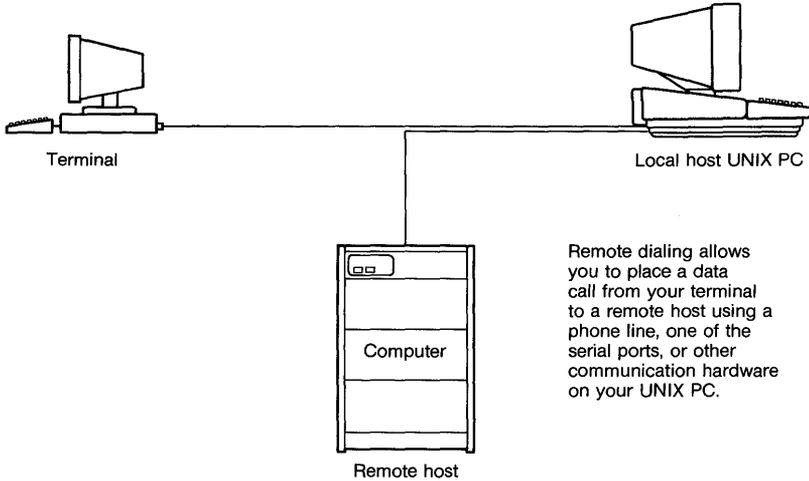
Remote dialing allows you to place a data call from your terminal to a remote host using a phone line, one of the serial ports, or other communication hardware on your UNIX PC.
