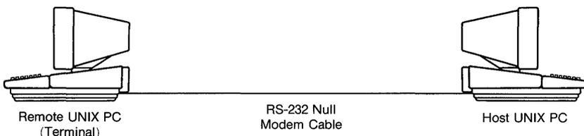
To attach a **UNIX** PC as a terminal to a host **UNIX** PC using the standard RS-232 port, set up the RS-232 port on the host **UNIX** PC for connection to a **COMPUTER** acting as a **HOST**.
