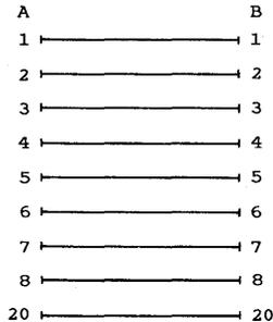
Use this type of cable when connecting 510 terminals and modems to the UNIX PC.
