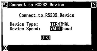
The terminal must be set up to run at the same baud rate as that entered in the Device Speed: field.
