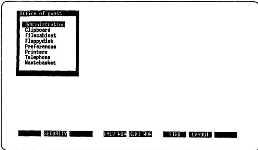
In a remote Office, window borders appear reversed and do not have icons. The screen keys are smaller than in the Office on a **UNIX** PC screen. See "Working from a Remote Terminal" later in this chapter for instructions on working in this Office using your particular model of terminal.
