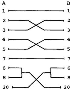
This type of cable is used primarily in terminal-to-UNIX PC connections. Turning off the terminal disconnects the line.
