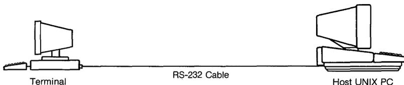
RS-232 cable connections are typically limited to 50 feet for proper operation at 9600 baud; however, longer cables can be used depending upon the environment and baud rates.
