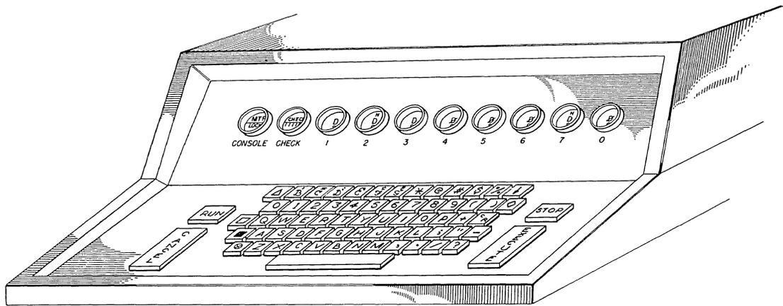
Figure 1. Keyboard and Indicator Lights on Honeywell 800 Console
