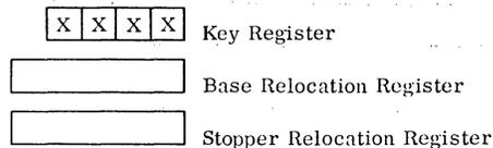
Figure 2. Program Control Registers within a Control Group; eight Control Groups are provided within the Model 8200 Word Processor.
