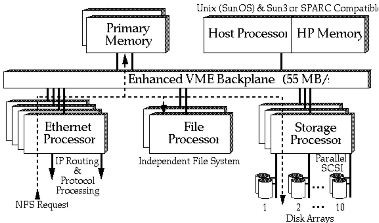
**Figure 2:** The NS 5000 functional multiprocessing I/O architecture. All network, file system, and storage processing is completely removed from the Unix host processor and performed instead by dedicated processors. Primary memory contains only file data and no instructions. The dashed line shows the data flow of an NFS read request through the system.
