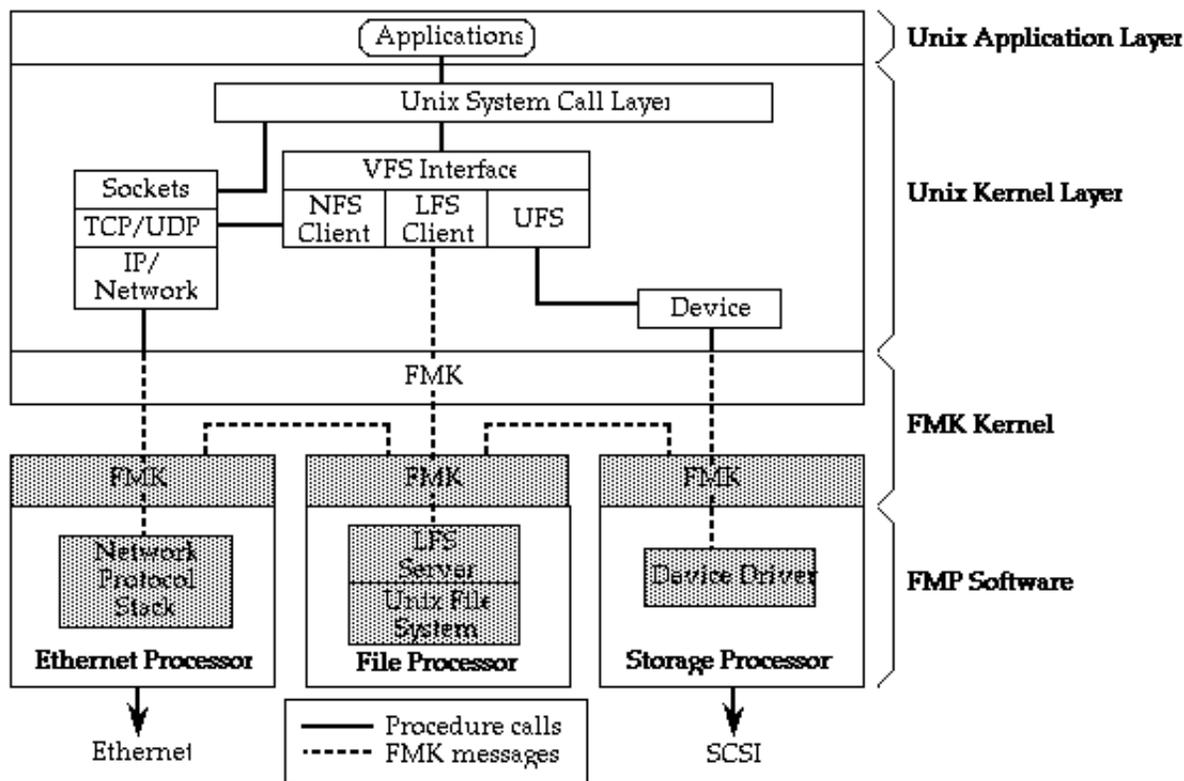
**Figure 7:** NS 5000 software structure. FMK executes on each hardware processor (large boxes). Solid connecting lines represent function calls. Dashed lines denote control paths using FMK messages. While the software structure is complex, the optimized NFS path is simple. The modules performing primary NFS processing are denoted *FMP Software* (shaded boxes).
