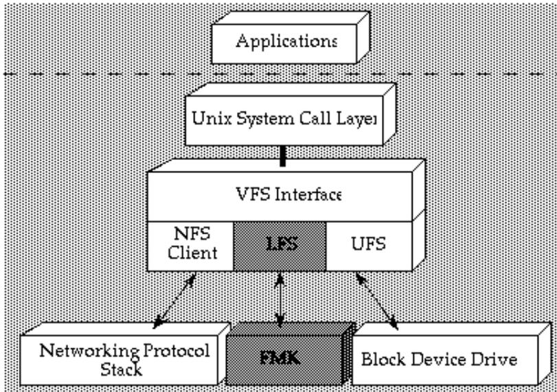
**Figure 5:** LFS control flow using VFS. LFS requests and responses are exchanged through message passing and not procedure calls. The FMK is a lightweight message-passing kernel used for interprocess communication between NS 5000 physical processors. From the FMK, LFS messages pass to the file processor (not shown).
