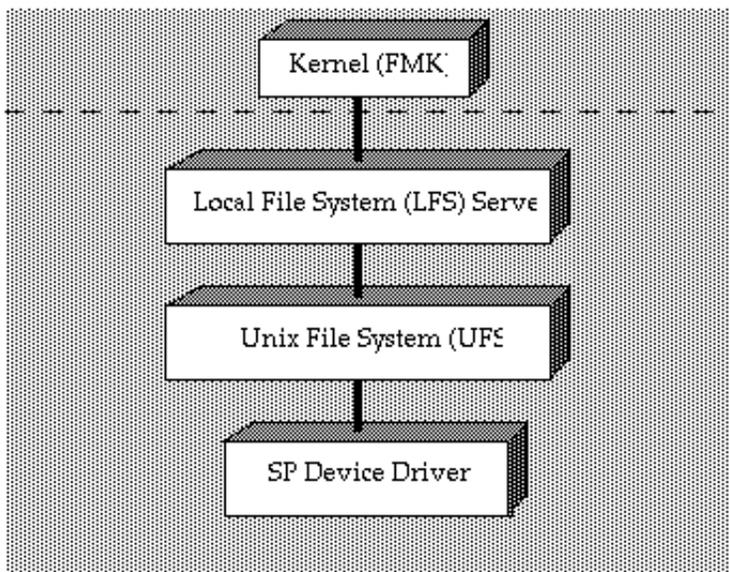
**Figure 6:** The architecture of the file processor software. FMK routes LFS requests to the LFS server. The LFS server makes UFS calls, and UFS calls *FP\_strategy*.
