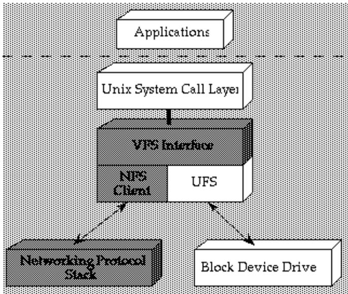
**Figure 4:** File system processing through the VFS interface. NFS and UFS are transparently supported through the VFS abstraction.
