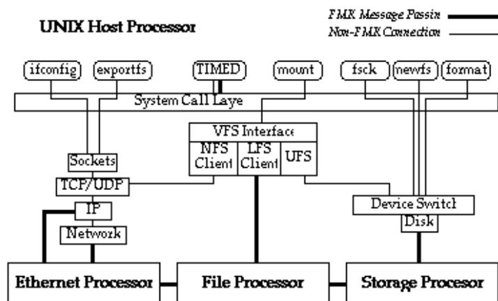
Figure 2: NS5000 software architecture using FMK for interprocess communication.
