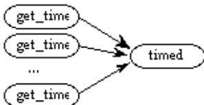
There is just one TIMED process so only one GET\_TIME or SET\_TIME message can be handled at a time. For many services, this is desirable. For instance, requests to a DMA service process *should* be queued for sequential processing because a DMA channel can handle only one request at a time. On the other hand, messages to a filesystem service process must not back up just because the current message is waiting for disk I/O.
