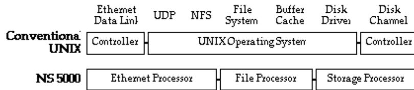
Figure 1: The distribution of NFS software functions using conventional and functional multiprocessing architectures.
