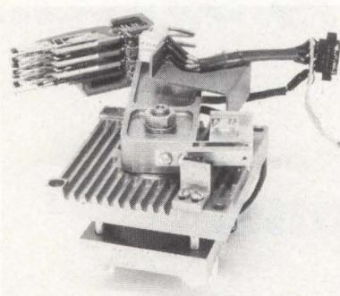
Small size and low cost are achieved in Okidata's series 3300 disc drives through use of a rotary head positioner. Heads are mounted directly on a rotating arm which moves across the disc surface much like a phonograph arm. This design does away with the typical head carriage and its mass, and eliminates precision rails and ball bearings.
