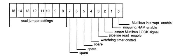
Figure 4-12 Multibus Adapter Misc Register Bit Map
