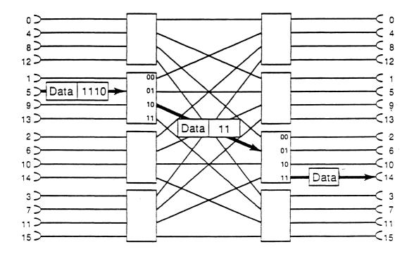
Figure 3-2 A Packet Moves through an 8-Node Switch
