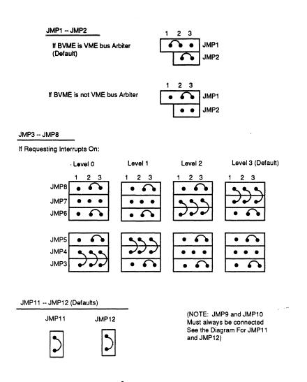
Figure 5-8 VME Bus Adapter Jumper Positions
