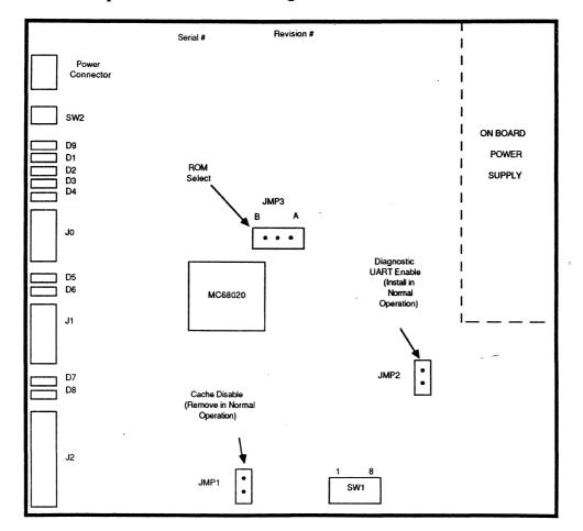
Figure 5-3 VME Node Controller Layout
