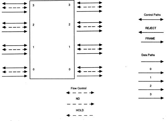
Figure 3-14 Base 4 Switch Node I/O Diagram
