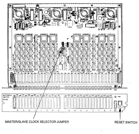
Figure 1–3 shows the Butterfly Plus switch card.
