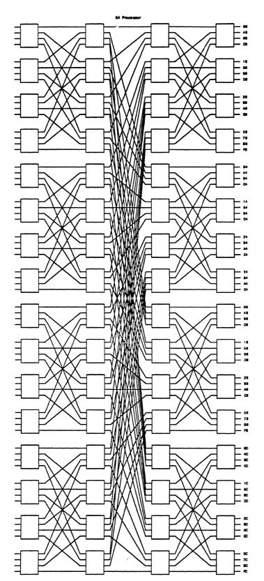
Figure 3-3 Switch for a 64-Processor Butterfly Plus
