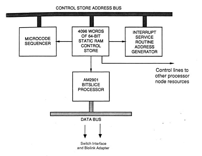
Figure 2-2 PNC Block Diagram
