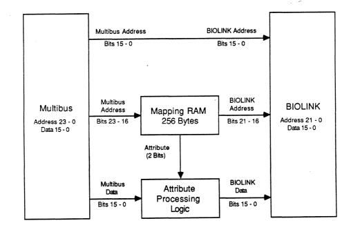
Figure 4-11 Mapping Multibus Addresses onto the BIOLINK
