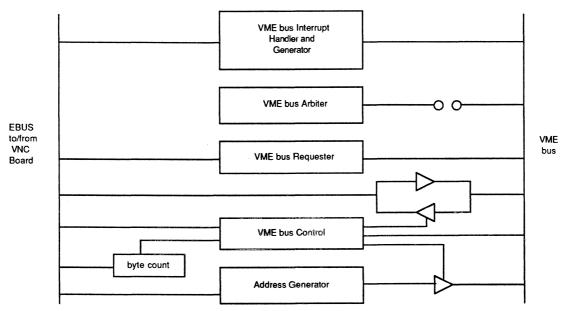
Figure 5-6 VME Bus Adapter Block Diagram
