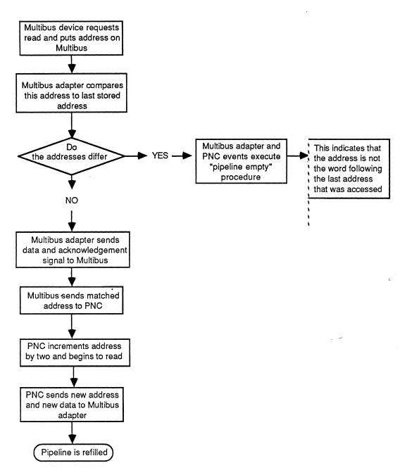
Figure 4-8 Pipeline Full Multibus Read
