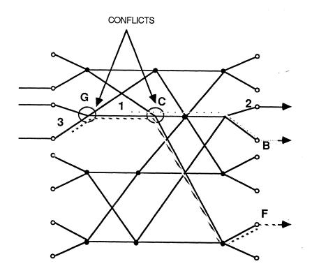
Figure 3-10 Secondary Blockage in the Switch
