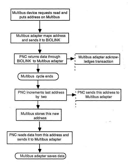
Figure 4-7 Pipeline Empty Multibus Read
