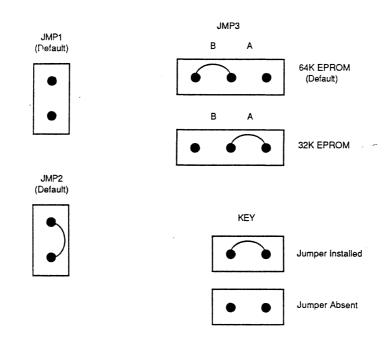
Figure 5-5 VME Node Controller Jumper Positions
