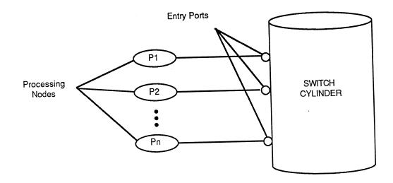
Figure 3-9 Switch as a Channel between Processor Nodes
