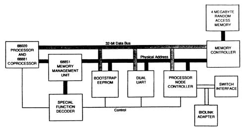
Figure 2-1 Processor Node Block Diagram
