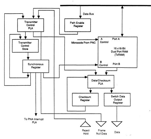
Figure 2-4 Switch Transmitter Block Diagram
