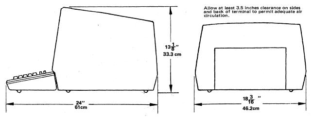
**Figure 2-1 Mounting Requirements**
