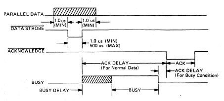
Figure 2-3 Parallel Port Timing
