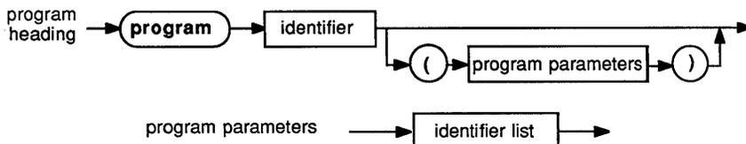
The program name is used to determine the default name of the code file in which to store the program's code when it is compiled to disk. You may override the default code file name with a `{%O <filename>}` compiler directive (see Appendix C, "Compiler Directives").
