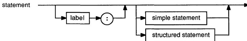
As you saw in Chapter 16, a label is either a digit sequence in the range 0 to 9999 or an identifier.
