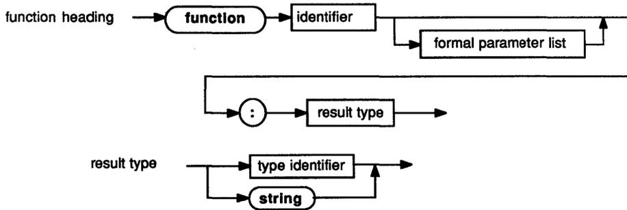
A **function** is activated by the evaluation of a **function call**. The **function call** gives the **function's** identifier and any actual parameters required by the **function**. A **function call** appears as an operand in an expression. When the expression is evaluated, the **function** is executed, and the value of the operand becomes the value returned by the **function**.
