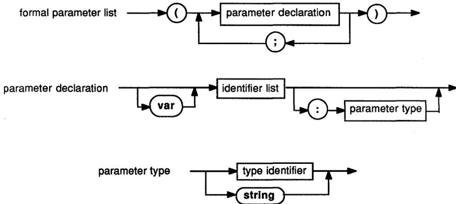
There are three kinds of parameters: *value parameters*, *variable parameters*, and *untyped variable parameters*. They are characterized as follows:
