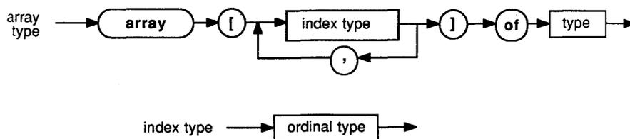
The index-types, one for each (unlimited) dimension of the array, specify the number of elements. The array can be indexed in each dimension by all values of the corresponding index-type; the number of elements is therefore the number of values in each index-type. Arrays may not occupy more than 32,767 bytes in total, and index-types may not be *LongInt* or subranges of *LongInt*.
