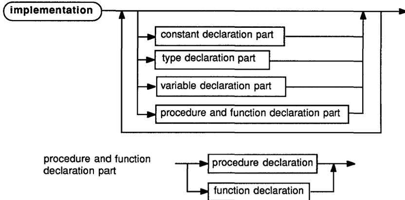
In effect, the procedure and function declarations in the interface-part are like **forward** declarations, although the **forward** directive is not specified. Therefore, these procedures and functions can be defined and referenced in any sequence in the implementation-part. While you repeat the procedure and function identifiers, you don't specify the formal parameter list for procedures and functions in the implementation-part.
