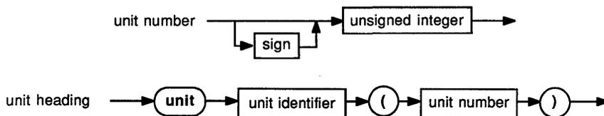
The unit name is used when referring to the unit in a uses-clause. Furthermore, it is used to determine the default name of the unit library file in which to store the unit when it is compiled to disk. You may override the default library file name with a `{%O <filename>}` compiler directive (see Appendix C).
