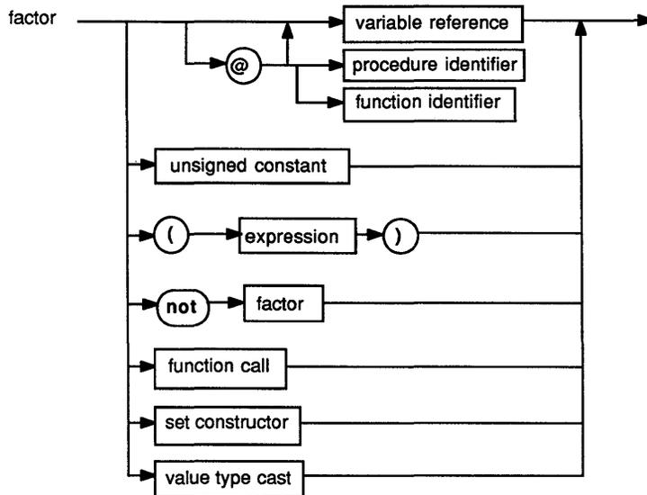
A function call activates a function, and denotes the value returned by the function (see “Function Calls” later in this chapter). A set constructor denotes a value of a set type (see “Set Constructors”). A value-type-cast changes the type of a value (see “Value-Type-Casts”). An unsigned constant has the following syntax:
