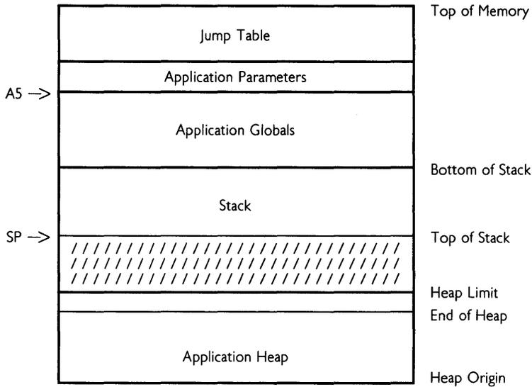
When an application starts up, the processor's A5 register is set to point to the boundary between the Application Parameters and the Application Globals. The Application Parameters and the Jump Table thus reside at positive offsets from A5 (above A5) and the Application Globals reside at negative offsets from A5 (below A5).
