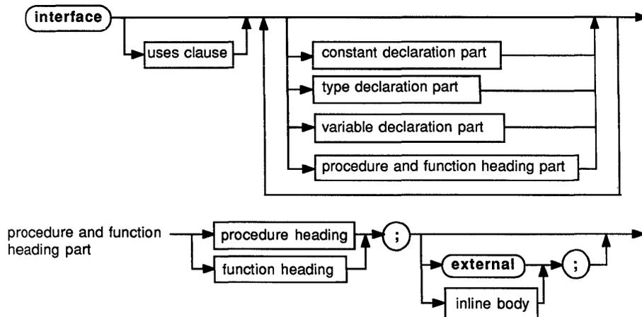
Unless a procedure or function is **inline** or **external**, the interface-part only lists the procedure or function heading. The block of the procedure or function follows in the implementation-part.
