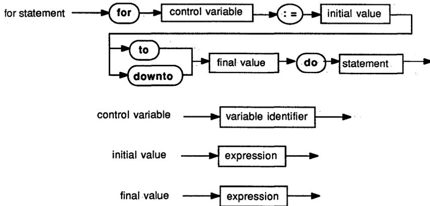
The control variable must be a variable identifier (without any qualifier) that signifies a variable declared to be local to the block containing the **for** statement. The control variable must be of an ordinal-type. The initial and final values must be of a type that is assignment compatible with the ordinal-type.
