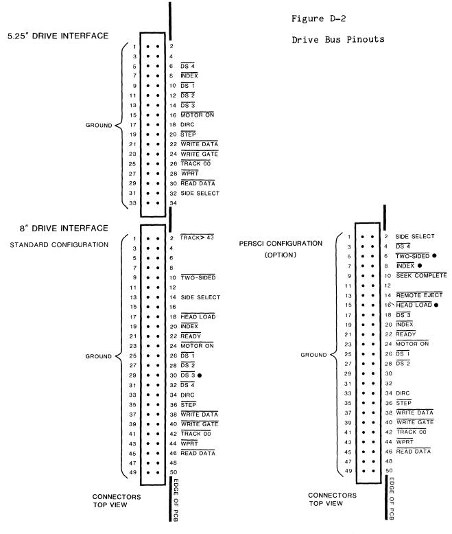
• These signals appear on the 8" drive bus in both configurations.
