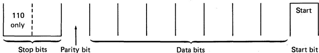
Figure 3-9. Asynchronous Format
