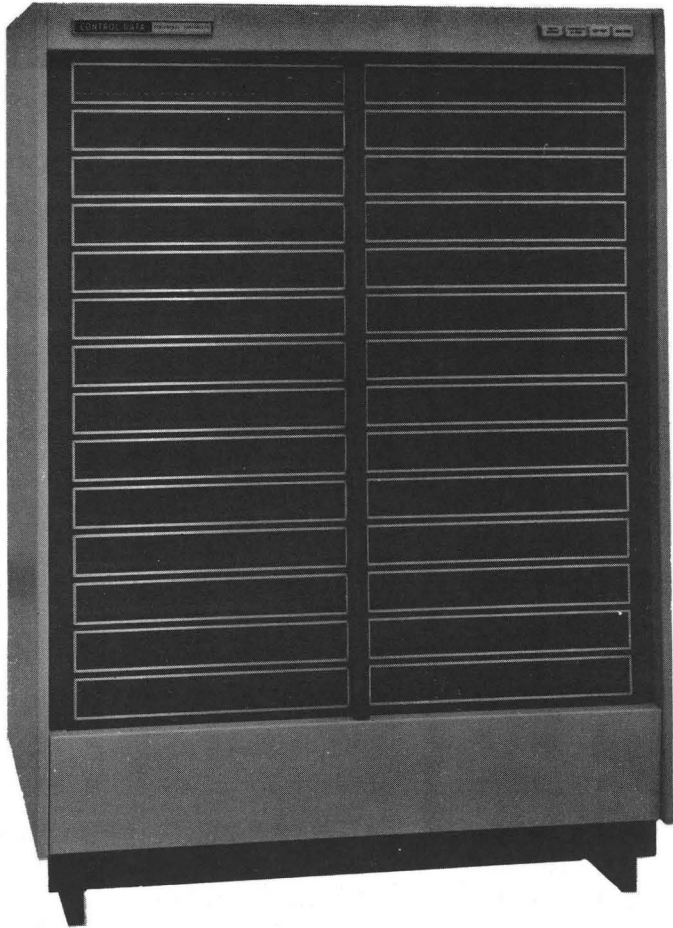
DRUM STORAGE CONTROLLER
