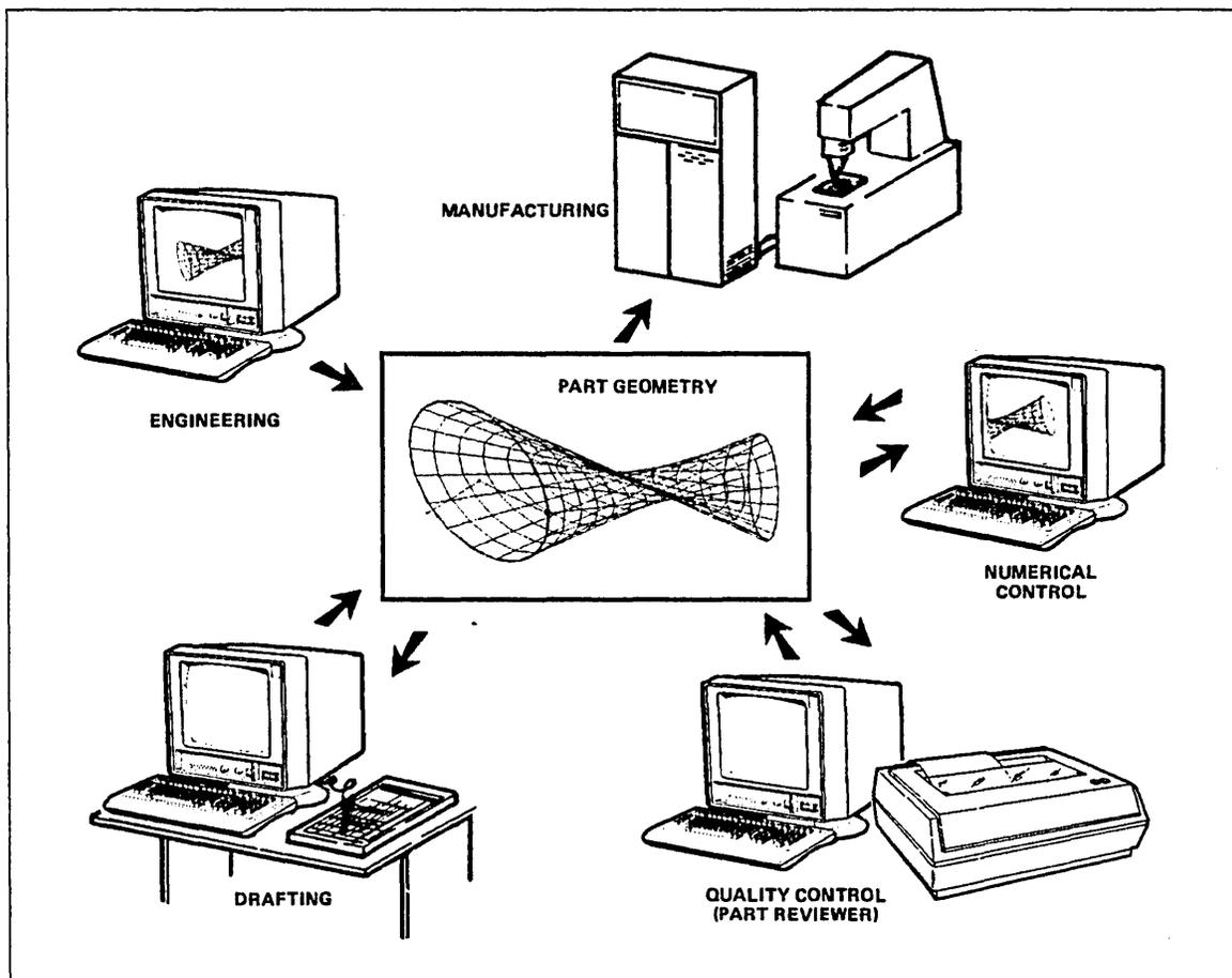
Figure 1-2. Sharing of Part Geometry
