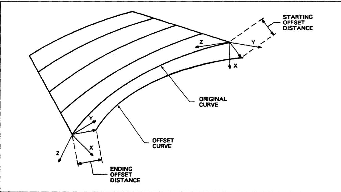
Figure 3-3. Offset in Variable Direction
