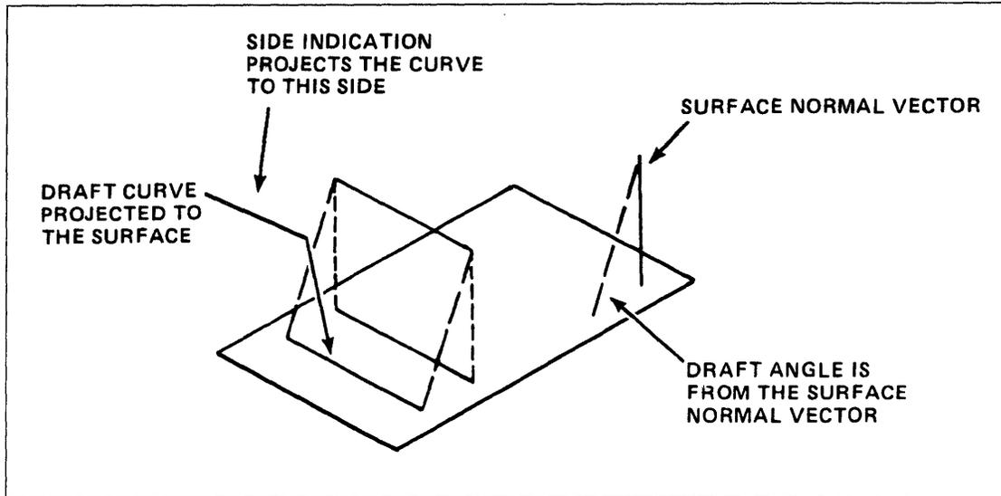
Figure 3-7. Draft Curve, Draft Angle, and Surface Normal Vector Examples
