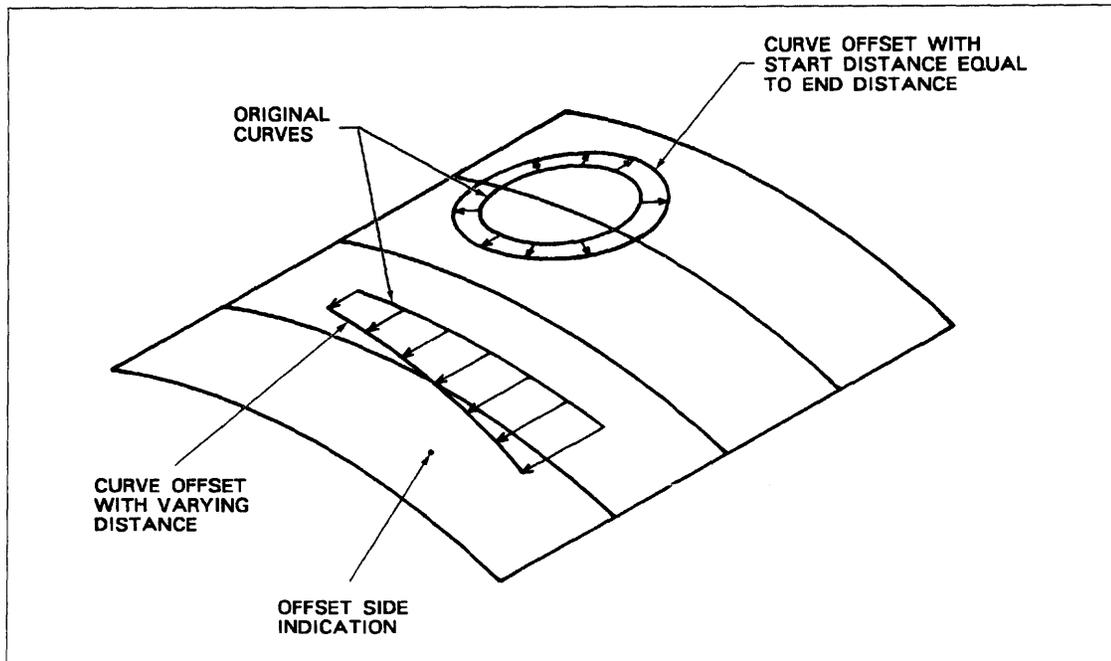
Figure 3-6. Offset Within the Surface
