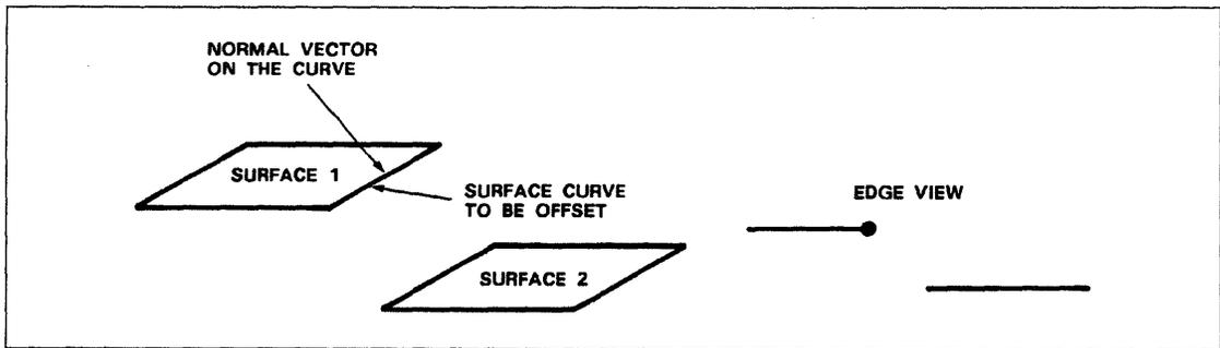
Figure 3-5. Inappropriate Use of the Normal Toward Second Surface Operation
