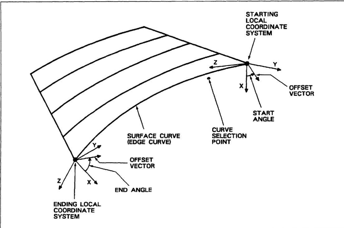
Figure 3-2. Local Coordinate Systems for Offset in Variable Direction
