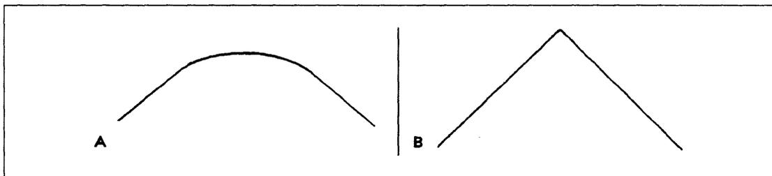
Figure 3-8. Curves Where the Tangent Vector: (a) Varies Continuously and (b) is Discontinuous at the Corner
