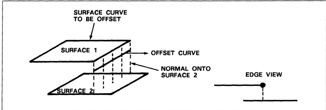
Figure 3-4. Appropriate Use of the Normal Toward Second Surface Operation
