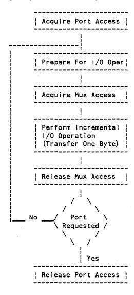
Common deck, COMPTMA, has been created which defines routines used to communicate with the two port mux. This deck should be referenced to obtain definitive information regarding use of the protocol defined below.
