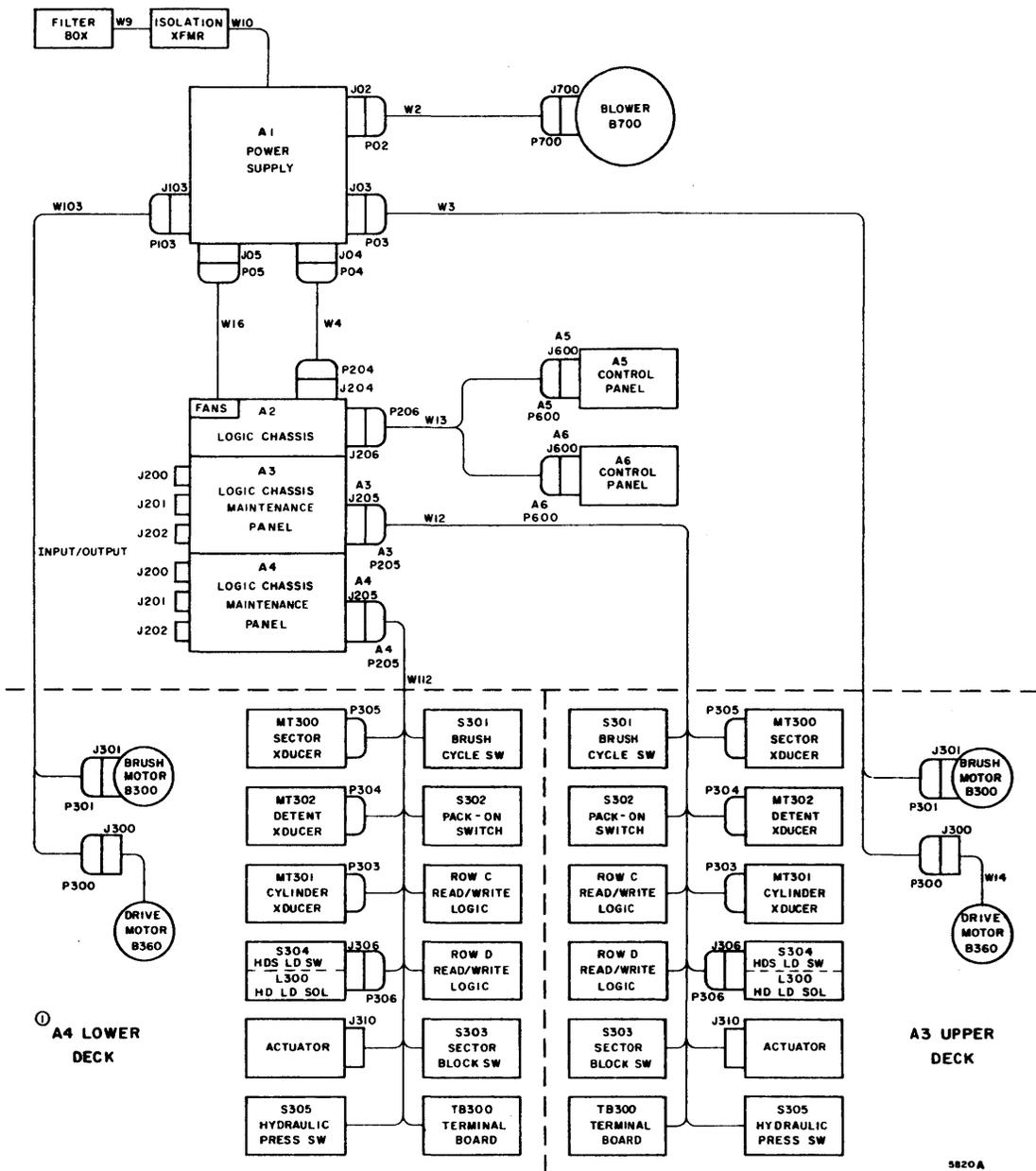
Figure 3-2. Cabinet Intracabling Diagram
