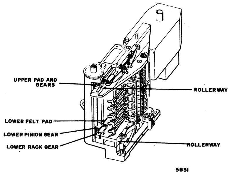
Figure 6-4. Carriage Lubrication
