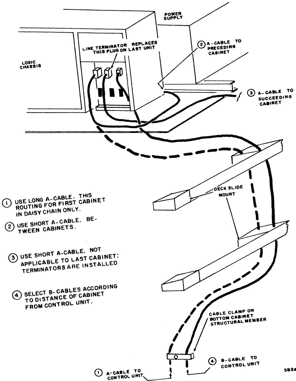
Figure 3-4. Intercabling Routing
