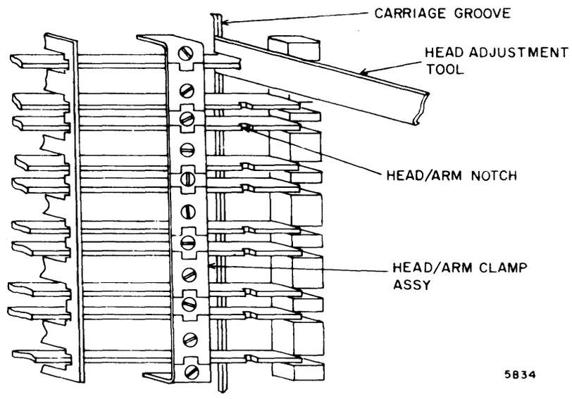
Figure 6-8. Head/Arm Assembly Adjustment
