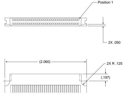
Figure 16. Non-shielded 68-pin SCSI device connector
