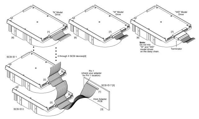
The drive device connector is a non-shielded 68-conductor connector consisting of two rows of 34 female pins with adjacent pins .050 inch apart. The connector is keyed by means of its shape (see Figure 16).
