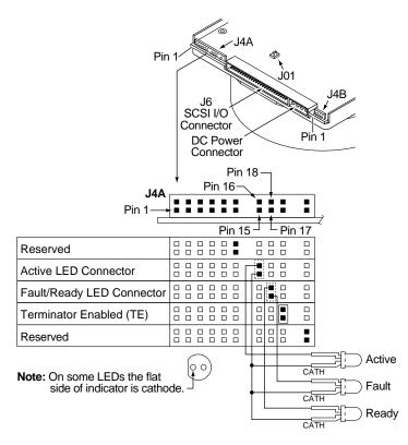
Figure 10a. J4A connections for Activity, Fault, and Ready LED indicators for all models
