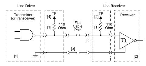
Figure 17. Single-ended transmitters and receivers
