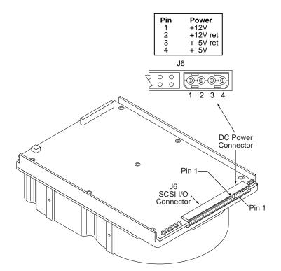
Figure 12. Physical interface for "N" model drives
