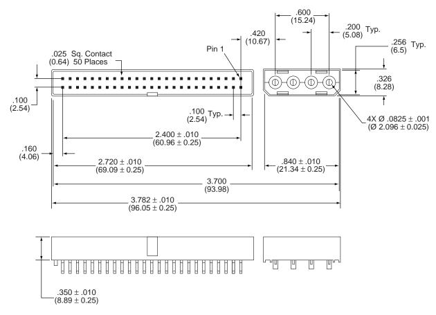
Figure 15. Non-shielded 50-pin SCSI device connector
