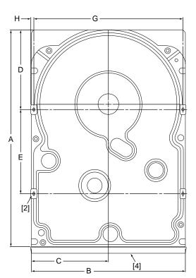
Figure 6. Mounting configuration dimensions for "N" models
