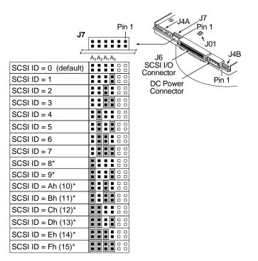
Figure 9b. ST423451 "WD" model auxillary remote cable ID select
