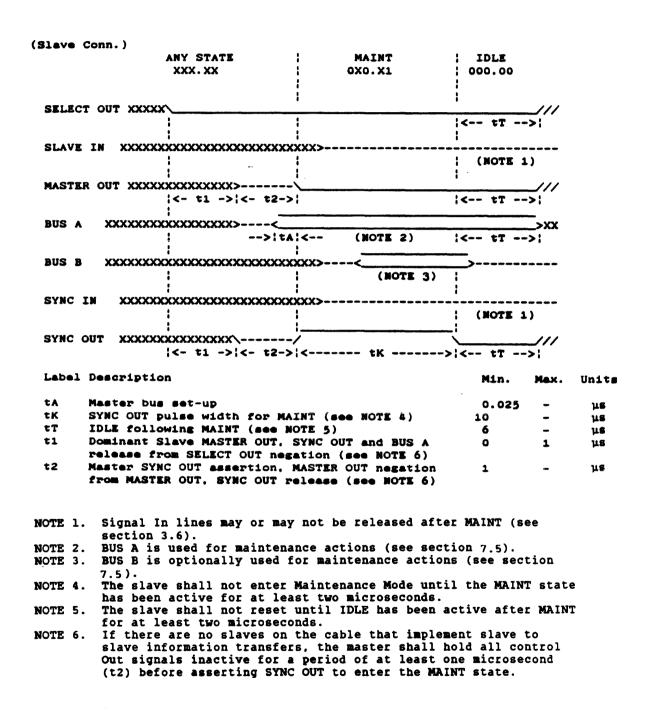
FIGURE 15. MASTER RESET TIMING
