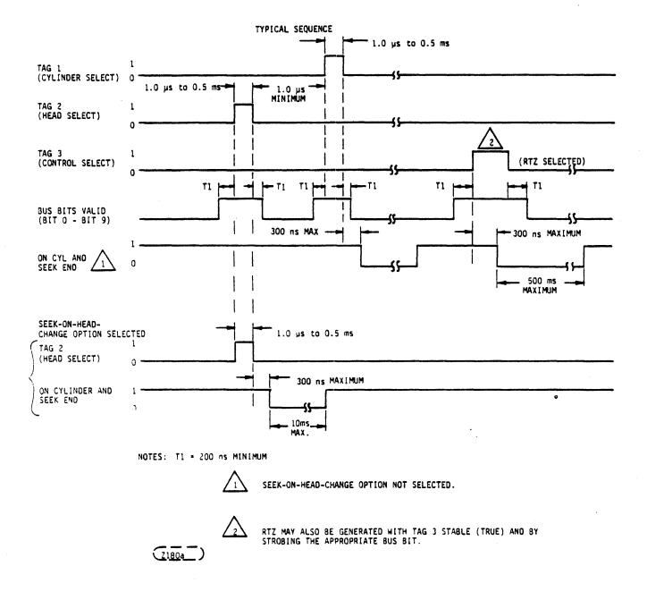
Figure 5.2-2. Tag and Bus Timing
