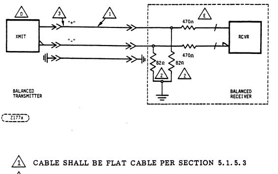
TERMINATOR RESISTORS ARE LOCATED ON DRIVE LOGIC CARD OR IN CONTROLLER. THESE SIGNALS MUST BE STAR CABLED.
