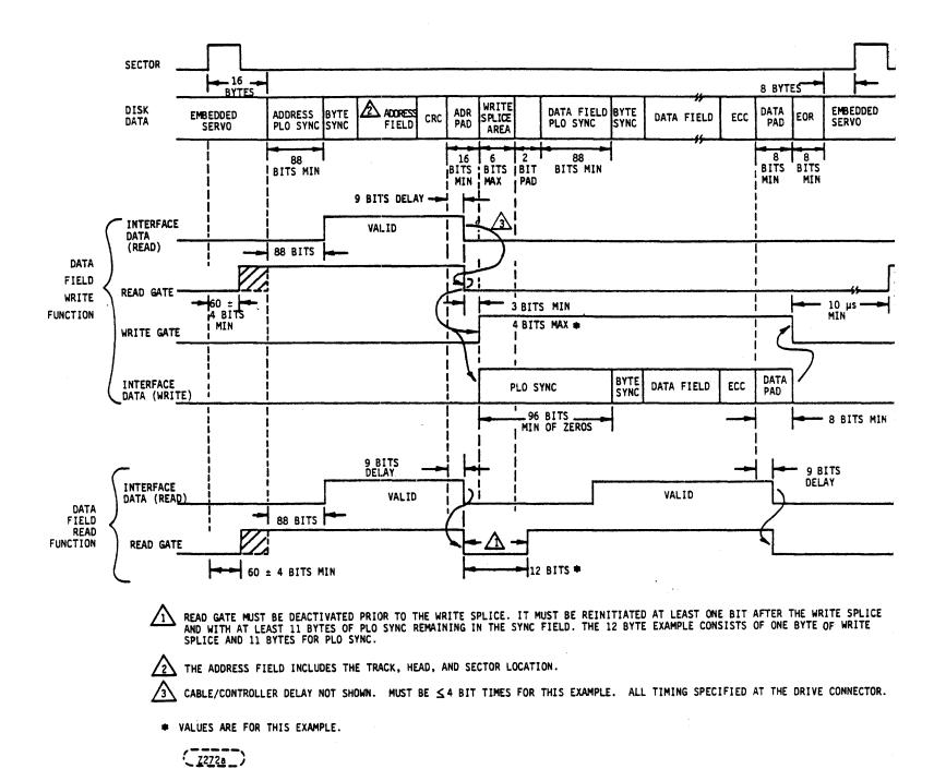
Figure 5.3-3. Typical Read/Write Timing
