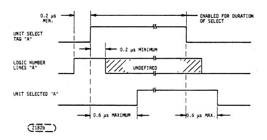
Figure 5.2-5. Logic Number Select and Timing Diagram
