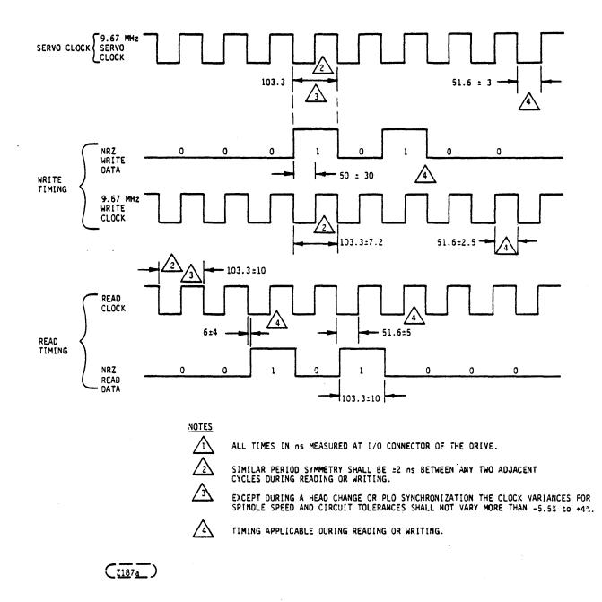
Figure 5.2-7. NRZ Data and Clock Timing
