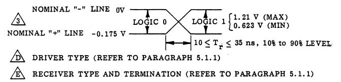
Figure 5.1-1. Typical Read/Write Data and Clock Transmitter and Receiver
