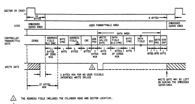
WRITING THE DATA AREAS ARE OPTIONAL. THESE AREAS ARE USEFUL TO VERIFY THE INTERGRITY OF THE SECTOR IF THE FORMATTER READ VERIFIES THESE AREAS AFTER A FORMAT OPERATION WHICH ALSO WRITES THE DATA AREAS. IF DATA FIELDS ARE TO BE WRITTEN, WRITE GATE MUST BE DEACTIVATED FOR A MINIMUM OF ONE BIT TIME AFTER THE ADDRESS PAD AND REACTIVATED 6 BITS PRIOR TO THE DATA FIELD PLO SYNC AREA.
