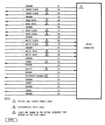
FIGURE 3-10. DATA CABLE CONNECTOR ASSIGNMENTS
