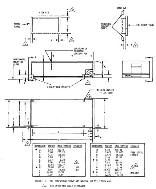
△4. CLEARANCE OF 0.75 INCHES (19.1 mm) MUST BE PROVIDED AT AIR EXITS.
