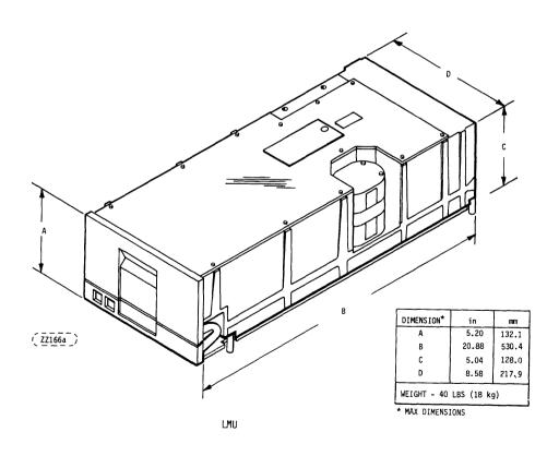
FIGURE 1.2. LMU PHYSICAL CHARACTERISTICS
