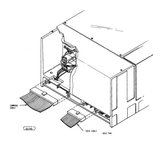
FIGURE 3-5. COMMAND/DATA CABLE CONNECTIONS
