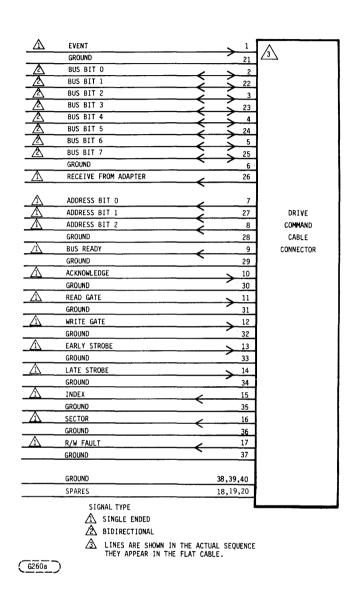
FIGURE 3-9. COMMAND CABLE PIN ASSIGNMENTS
