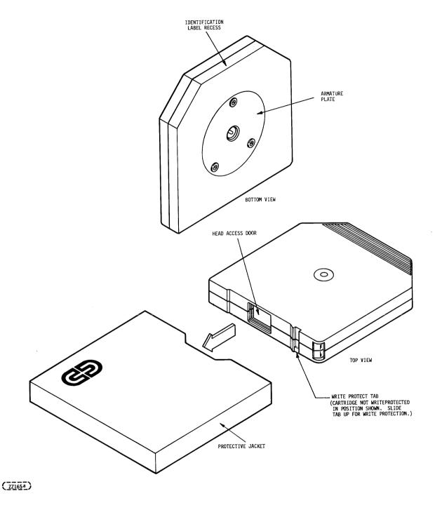
FIGURE 2-3. DISK CARTRIDGE SHOWING PROTECTIVE JÄCKET AND WRITE PROTECT TAB
