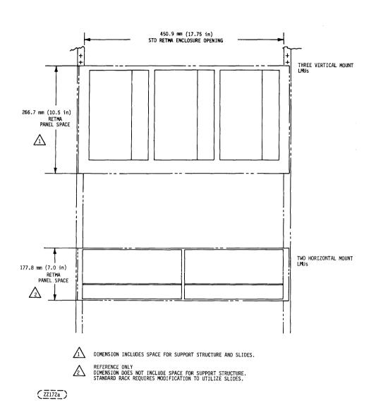
FIGURE 3-3. EXAMPLE LMU CONFIGURATIONS
