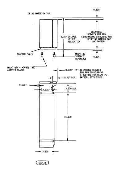
FIGURE 3-2. LMU VERTICAL MOUNTING DIMENSIONS
