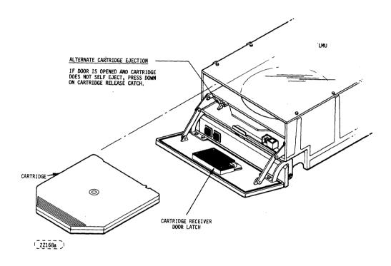
FIGURE 2-2. DISK CARTRIDGE; CARTRIDGE INSTALLATION AND REMOVAL
