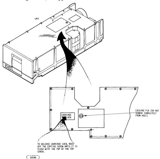
FIGURE 3-11. CARRIAGE LOCKING PIN
