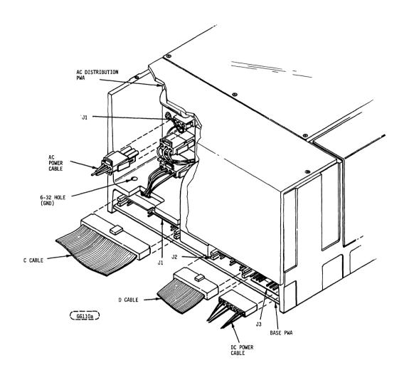
FIGURE 3-6. AC AND DC CABLING
