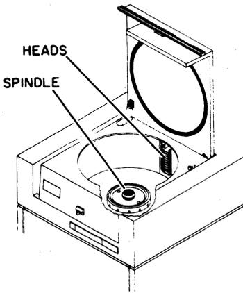
to the figure, locate the spindle and heads.
