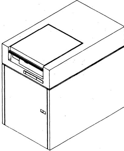
Use this section as a guide in locating essential parts of your disk drive. First, find the operator control panel (on the upper lefthand part of the front surface).
