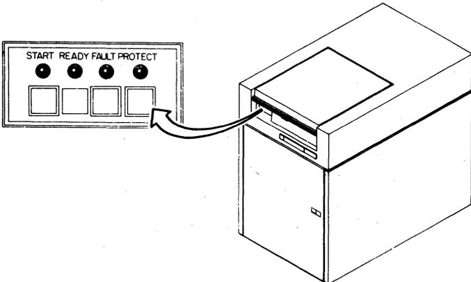
The operator control panel contains the controls and indicators used to operate the drive. The panel shown above is a typical one; the panel on your drive may be layed out differently. The individual parts on the operator control panel are discussed in detail in the "Controls and Indicators" section.
