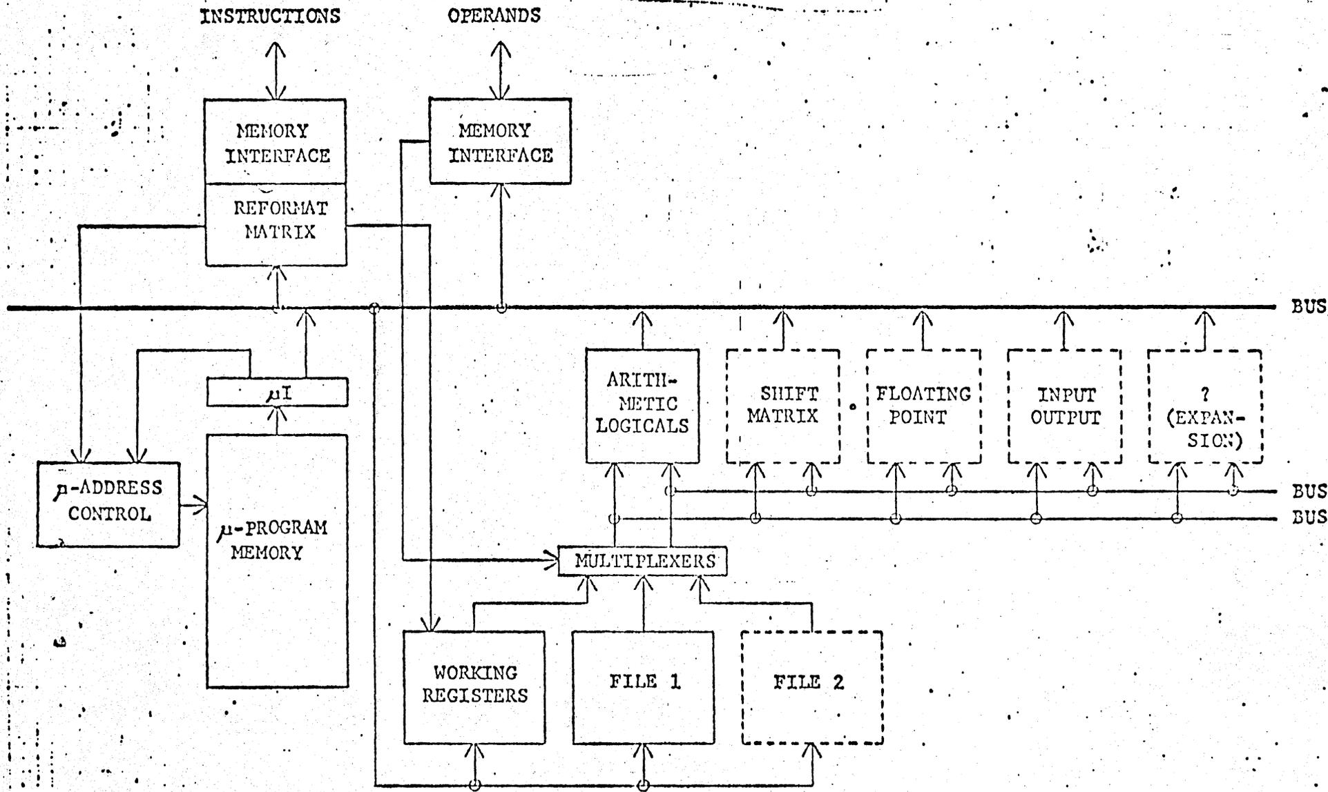
Figure 3-4. AMPP Simplified Block Diagram of Processor
