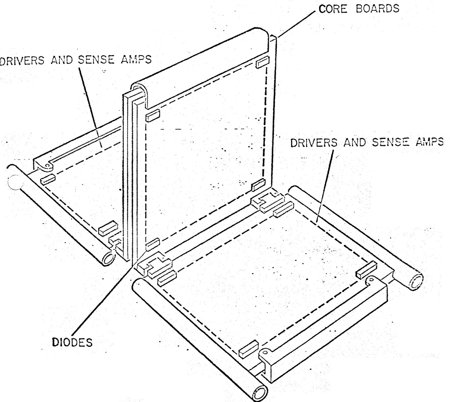
Figure 3-2. Memory Module-Component Access
