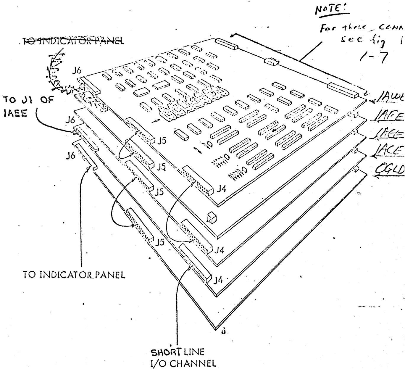
Figure 1-6. Cable Connections (Front View)
