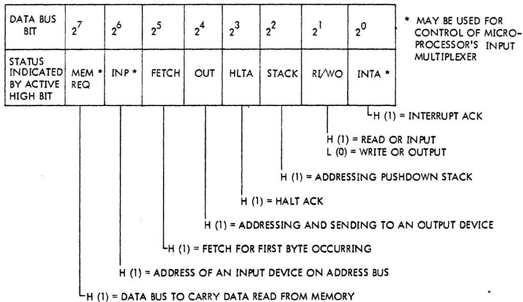
Figure 4-10. Microprocessor Status Byte
