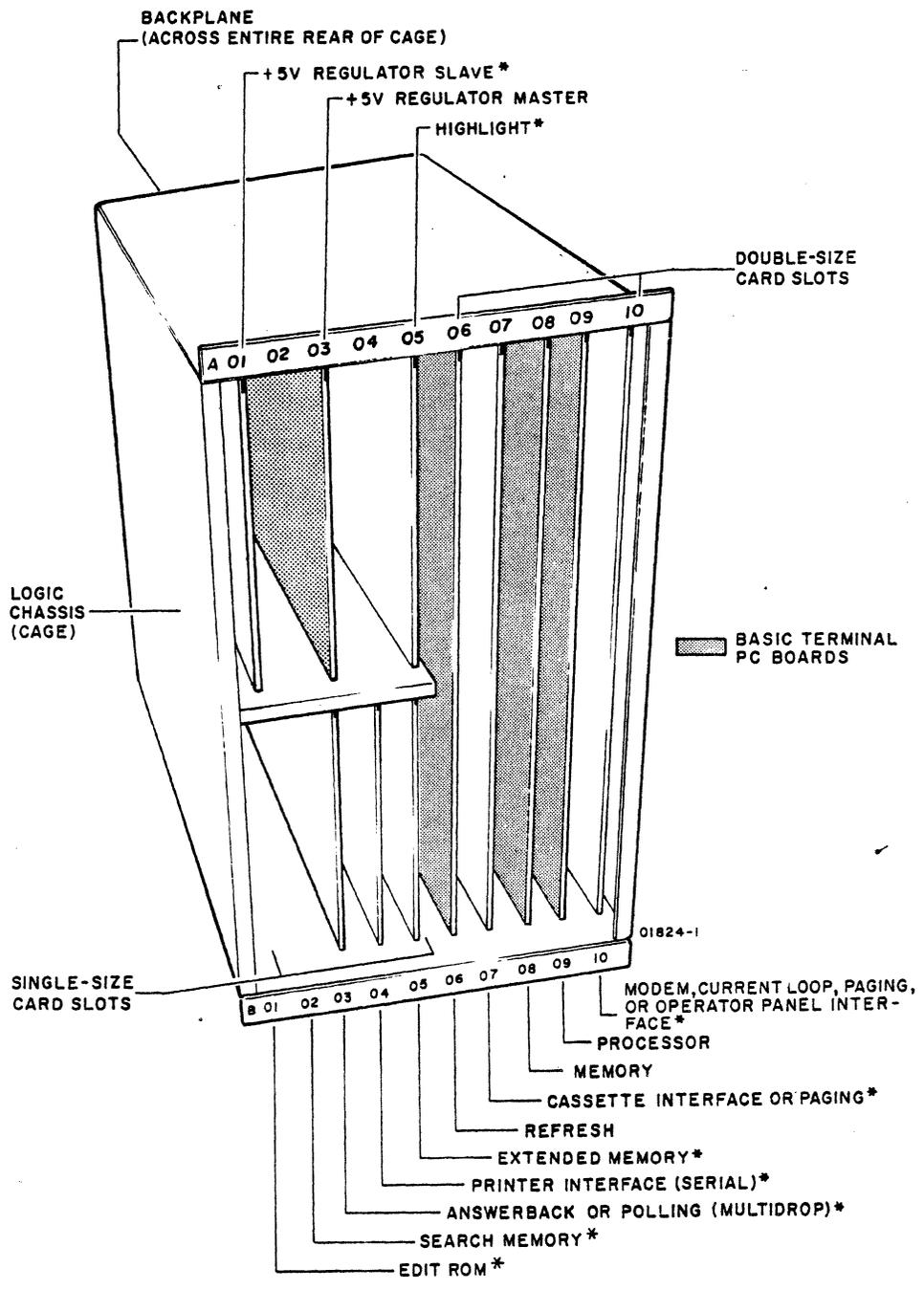
\* OPTIONAL CARDS. ONE +5V REGULATOR ALWAYS REQUIRED AT A03, BUT AN ADDITIONAL ONE MAY BE PRESENT AT A01 TO SUPPLY ADDITIONAL POWER REQUIRED FOR OPTION CARDS.
