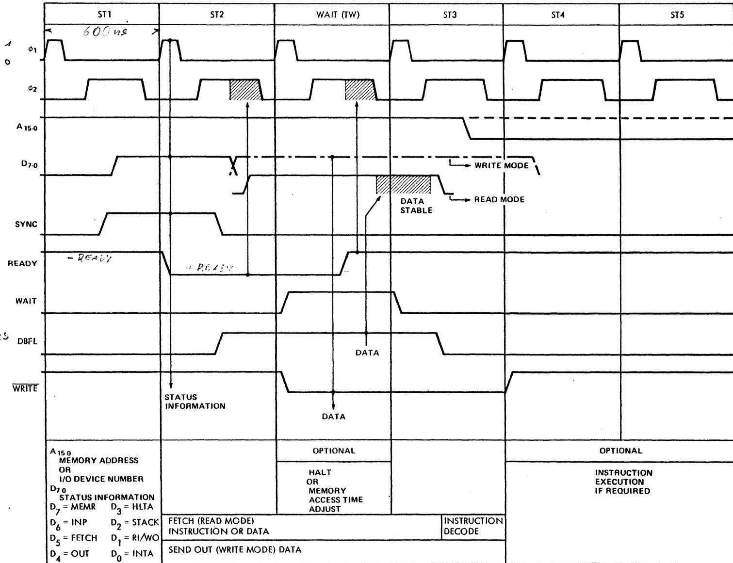
Figure 4-8. Microprocessor I/O Timing for Instruction Cycle
