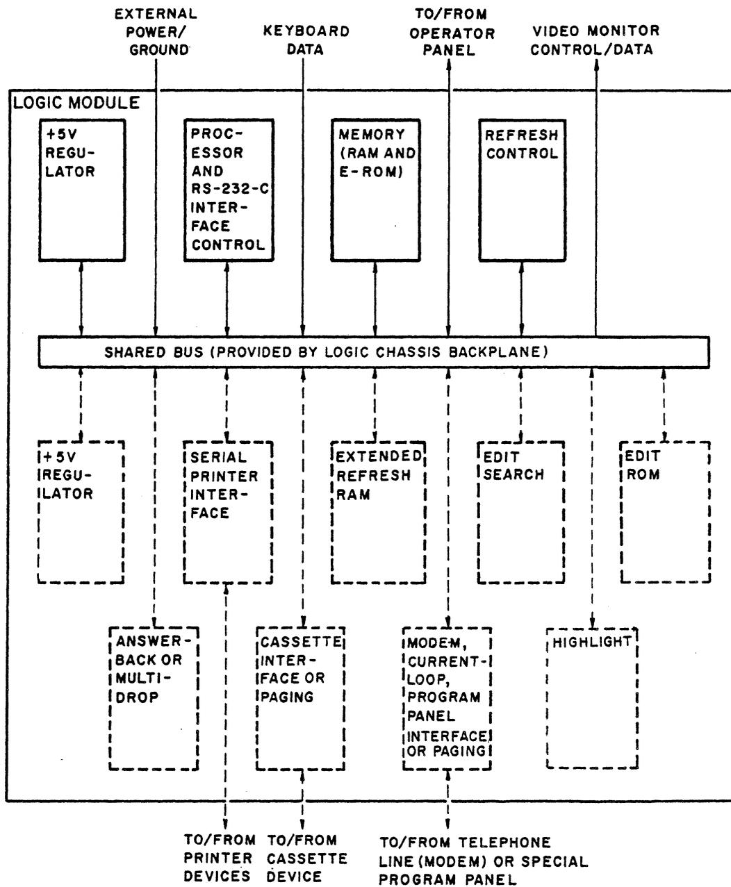
NOTE: SOLID LINES SHOW BASIC LOGIC MODULE FUNCTIONAL SUBASSEMBLIES. BROKEN LINES SHOW OPTIONAL FUNCTION CARDS.
