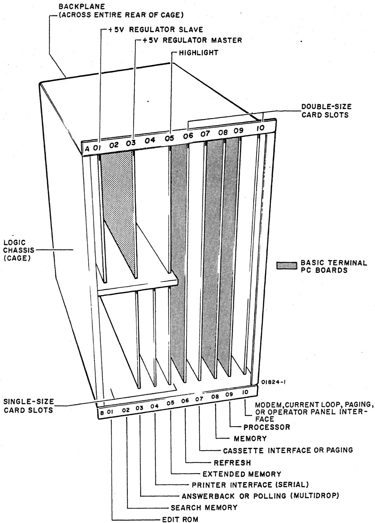
Figure 4-1. Logic Module Physical Architecture
