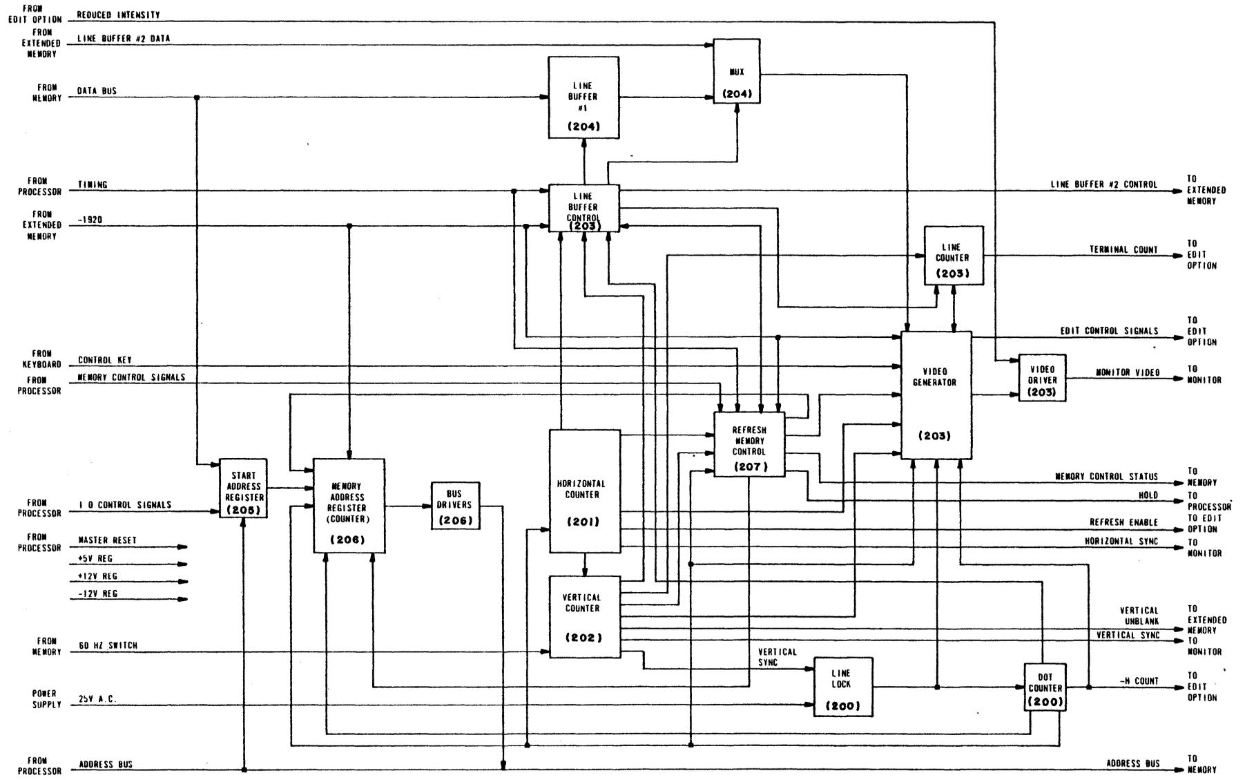
NOTE: DESIGNATIONS IN PARENTHESES, E.G., (000) REFERENCE THE LOGIC DIAGRAMS WHICH SHOW THE DETAILED CIRCUITS.
