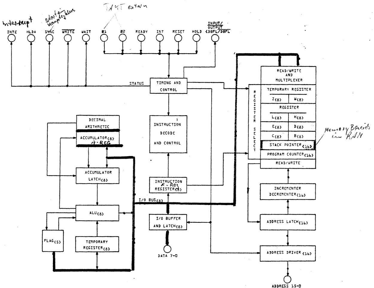
Figure 4-6. Microprocessor Chip Functional Diagram
