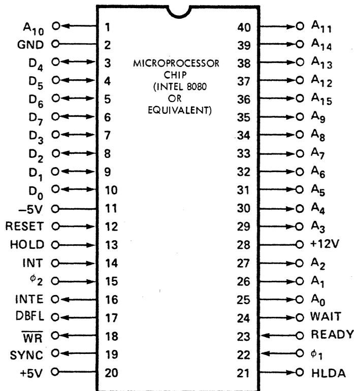
Figure 4-7. Microprocessor I/O Signals
