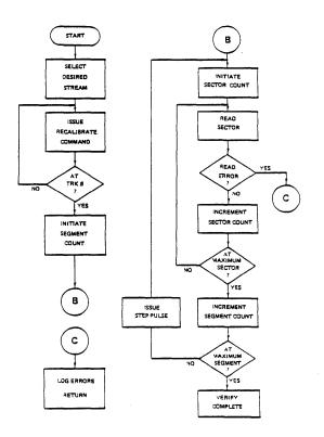
Figure 9-7. Verification Pass Flowchart
