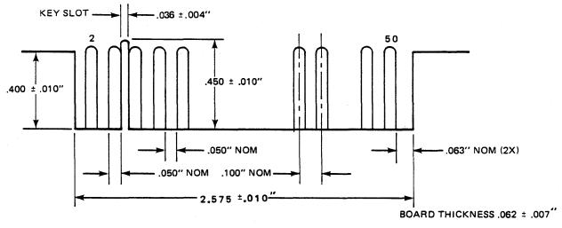
Figure 6-3. J1 Interface Connector Dimensions - SA850
