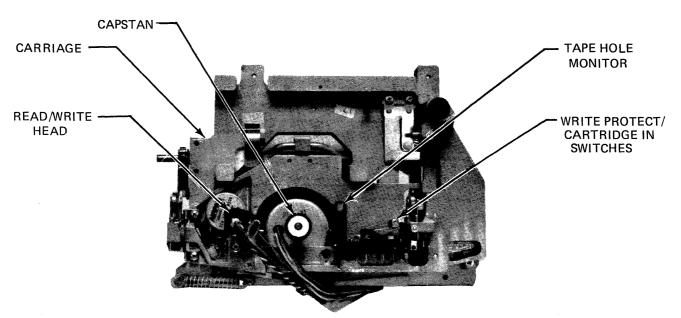
Figure 3-2. Component Location Layout
