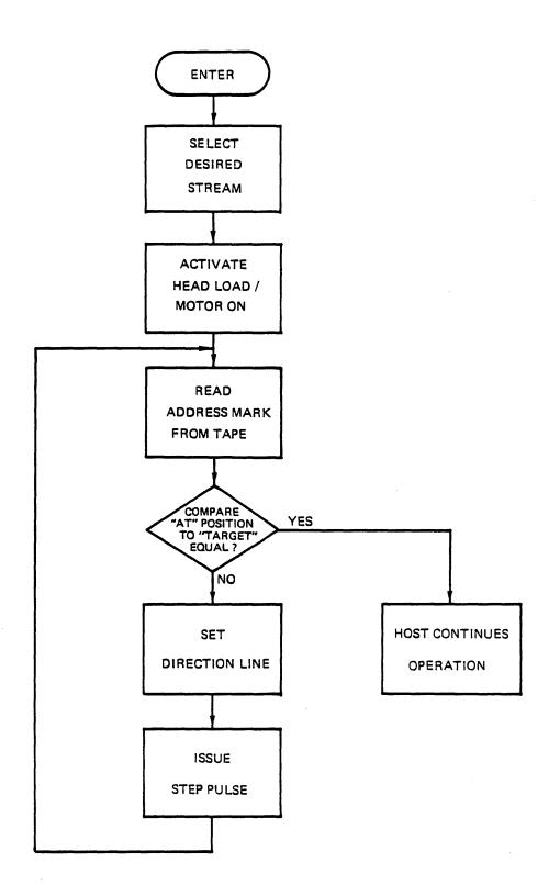
Figure 4-3. Stream Access Flowchart
