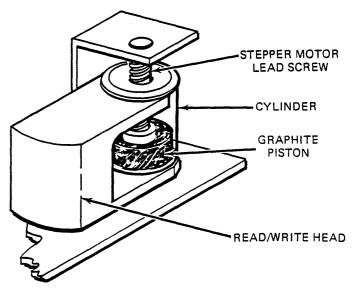
Figure 3-3. Read/Write Head Assembly
