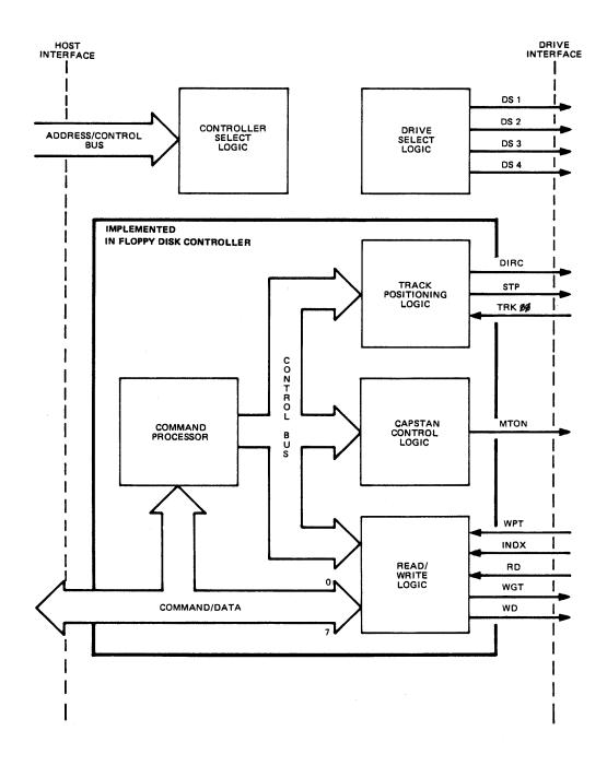
Figure 9-2. Typical Floppy Disk Host Controller
