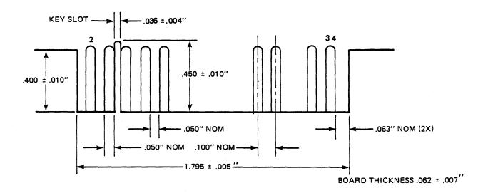
Figure 6-2. J1 Interface Connector Dimensions - SA450
