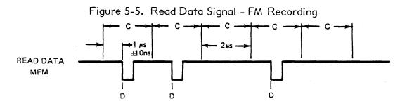
D = Data Pulse =  $300 \pm 50$  ns Bit Cell Time = 2  $\mu$ s
