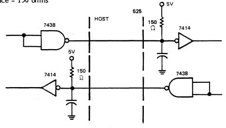
Figure 5-4. Interface Signal Driver/Receiver
