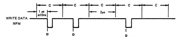
D = Data Pulse = 150 ns min, 1  $\mu$ s max. Bit Cell Time = 2  $\mu$ s  $\pm$ 10 ns
