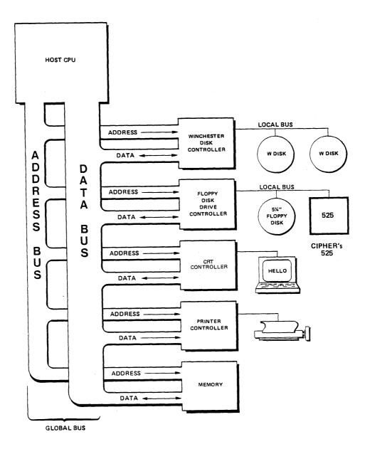
Figure 9-1. Typical Host System (Block Diagram)
