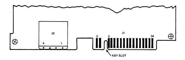
Figure 6-1. 525 Interface Connectors - SA450
