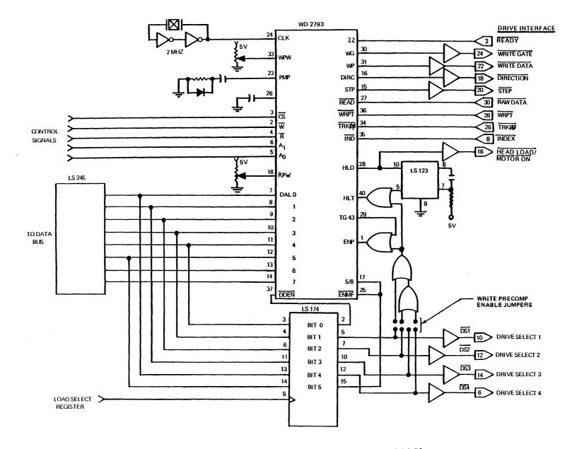
Figure 9-3. 525 Controller Example - SA450
