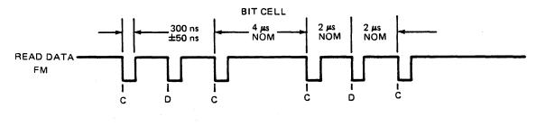
C = Clock Pulse =  $300 \pm 100$  ns Bit Cell Time = 4  $\mu$ s  $D = Data Pulse = 300 \pm 50 ns$
