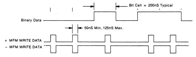
FIGURE 12. MFM WRITE DATA TIMING.
