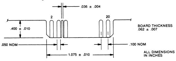
FIGURE 6. CONNECTOR DIMENSIONS
