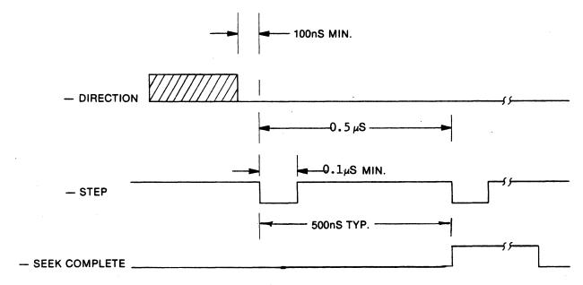
FIGURE 9. STEP PULSE TIMING
