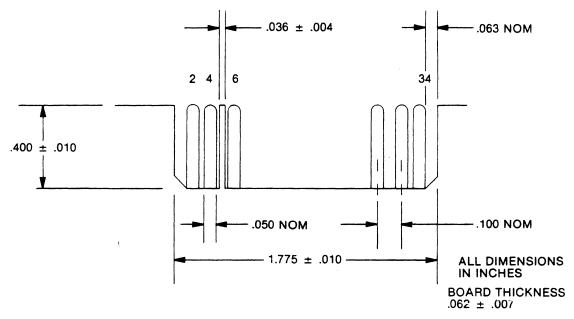
FIGURE 5. J1 CONNECTOR DIMENSIONS
