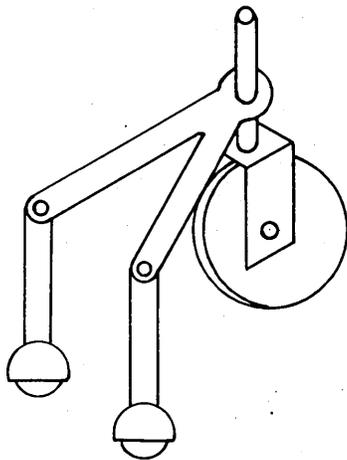
Now if a force  $F$  which is not too great is applied to this tricycle in a direction not perpendicular to the front wheel, then as in the case of the integrating wheel described in Section 3 of Chapter I above, the tricycle will move in a path to which the front wheel is tangent. The component of  $F$  which is parallel to the axle of the wheel is
