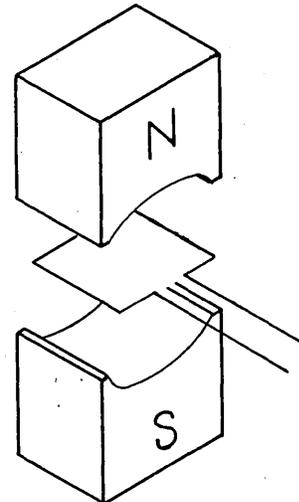
sume that the field is uniform and that the wire loop lies in a plane. If  $\theta$  is the angle of rotation of the loop from a fixed position of maximum flux. then  $\phi = A \cos \theta$  and  $e = k\dot{\phi} = -kA \sin \theta \frac{d\theta}{dt}$ .
