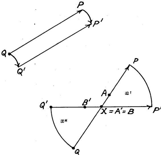
of these, the new position  $Q'P'$  does not intersect  $QP$ , in the second case, it does. In the first case the area is readily defined. The point  $P$  describes an arc  $P'P$  and the point  $Q$  an arc  $Q'Q$  and these together with the initial and final position of the line segment enclose an area which is given by the formula
