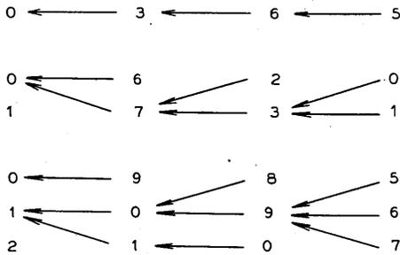
4. The above process of "splitting" the multiplication table is the basis of the "Millionaire" machine, as proposed by the French inventor, Bollee. We describe the essential idea in terms of our previous example. (Our description differs slightly from the precise situation.) Again, we wish to multiply 365 by 132. The machine has three feeds, one for the units in the multiplication table, one for the tens in the multiplication table and one for the tens transmission.
