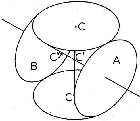
Geometrically, the motion of the bevel gears is equivalent to the motion of non-slipping right circular cones or frustums of cones. We can even replace each gear by a disk contingent to other disks, the disk representing a cross-section of the cone perpendicular to the axis. These disks must rotate without slipping.
