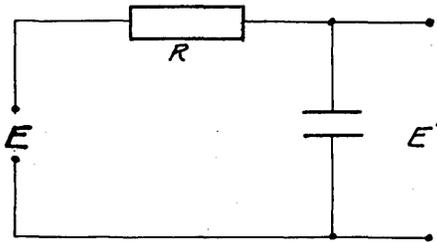
then the voltage  $E'$  across the condenser is  $q/C$  where  $C$  is the capacity of the condenser. The current  $i$  through the resistance is  $\frac{dq}{dt}$  and thus the input voltage
