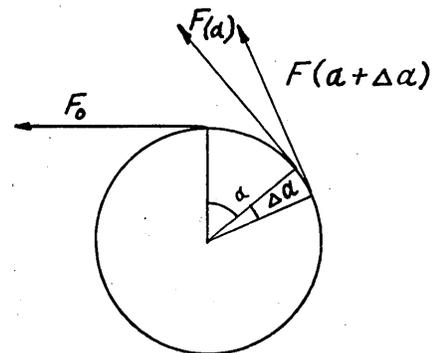
for this point of first contact and an arbitrary radius. Then the longitudinal tension in the band is a function  $F(\alpha)$  of this angle.
