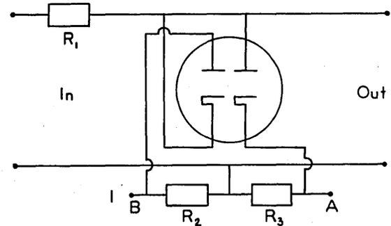
Normally no current flows in resistors  $R_2$  and  $R_3$  and the output is essentially shorted through the diodes and  $R_2$  and  $R_3$ . If a current flows through  $R_2$  and  $R_3$  from A to B, then each diode plate is below its cathode and the diode is effectively a large resistance and the output voltage is a considerable fraction of the input voltage.
