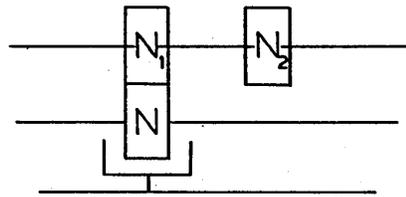
The full possibilities of shift and clutch gear arrangements can only be realized when the differential is introduced. The symbol for a differential most widely used is
