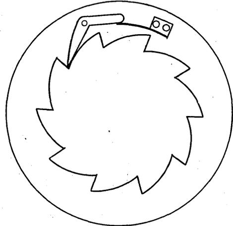
opposite direction, i.e., counter-clockwise, the ratchet is supposed to slip over the smooth part of the tooth and the rear wheel is supposed to remain stationary under the expected load conditions.
