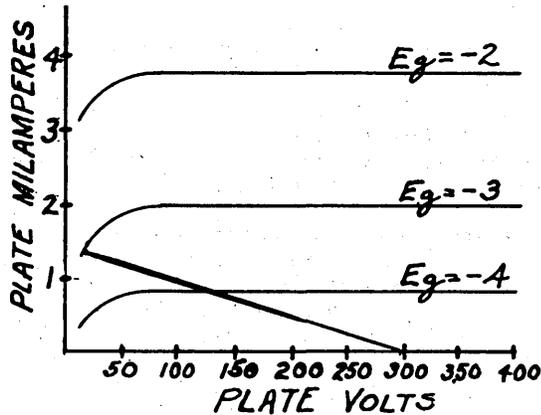
If we wish to use a system in which the unit of current is .001 amperes, then the unit of resistance is 1000 ohms. Hence in this system  $Z = 2 \cdot 10^2 = 200$  units. If we wish our voltage unit to be 50 volts we must give  $Z$  the value 4. (Another way of getting the above is to notice that in a milampere 50 volt system the unit of resistance is 50,000 ohms.) Consequently the slope is  $\frac{1}{4}$  and we draw this line.
