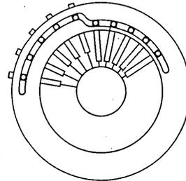
The Ohdner wheel is a similar feed, only here we have retractable teeth instead of teeth of different length. The number of teeth which protrude is set before addition. This, of course, is considerably more compact than the previous arrangement. (Cf. Galle, *loc. cit.*, pp. 33 and 34, figures 33 and 34.)
