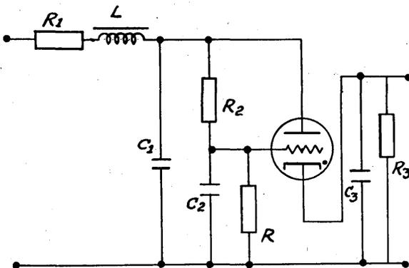
cuit, the two condensers  $C_1$  and  $C_2$  charge until  $C_2$  reaches the potential at which the "trigger grid" of the gaseous triode will initiate a discharge. Then  $C_1$  will discharge through the tube and  $C_2$
