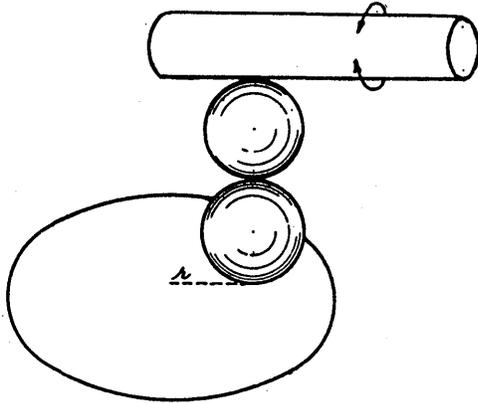
easily seen to be transmitted to the upper ball and the latter in turn transmits it to the cylinder and if  $\beta$  is the amount of rotation of the cylinder,  $\alpha$  that of the disk and  $r$  the displacement of the point of contact from the center of the disk, then  $d\beta = r d\alpha$ .
