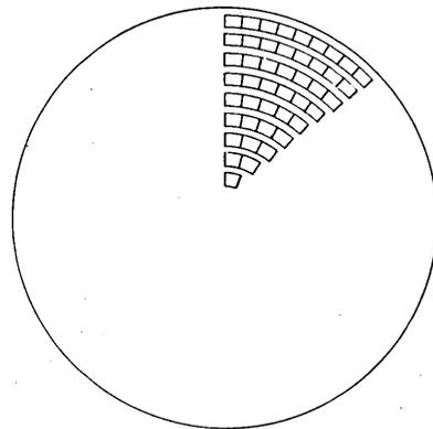
Another feed similar to the Leibnitz wheel is the feed of the "Gauss" machine. (Cf. Galle, *loc. cit.*, pp. 34, 35, 36.) Here we have a disk instead of a cylinder which has a different number of teeth at varying distances from the center. If the disk is revolved once, each feed wheel comes in contact with a varying number of teeth depending upon its position.
