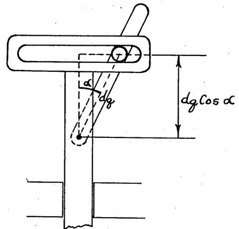
The multiplication by  $d_q$  is obtained by varying the length of the segment. Addition is by means of an endless chain.
