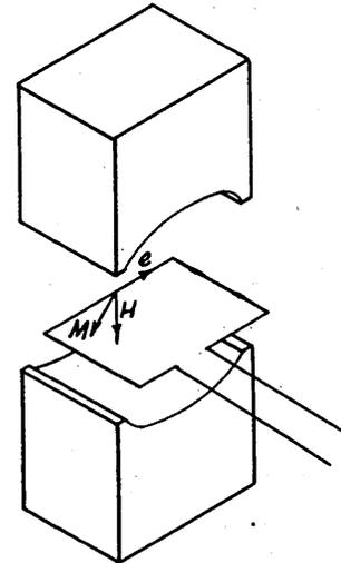
tion of the magnetic field  $\mathbb{H}$  on an element  $dl$  of length of the wire. Let  $m$  denote the motion of the element. Then the voltage rise  $e$  is a vector which is given by the equation  $e = m \times \mathbb{H}dl$ , i.e.,  $e$  is perpendicular to both  $m$  and  $\mathbb{H}$  and has size  $m\mathbb{H} \sin \theta' dl$  where  $\theta'$  is the angle between  $m$  and  $\mathbb{H}$ .
