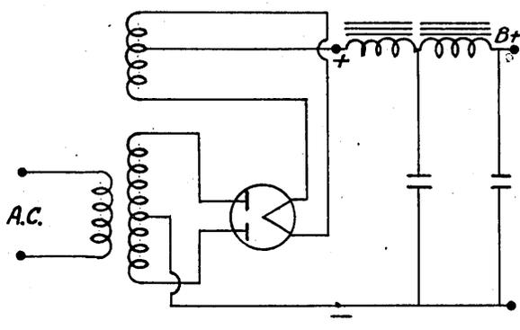
are called "filter chokes" and may have values from 8 to 30 henries, the condensers are usually electrolytic condensers of 8 to 30 microfarads. The inductances have resistances of about 200 ohms. The condensers should be of the correct "working voltage" which is, in general, the peak output voltage of the rectifier. (Sometimes it is higher if the inductances are too low.)
