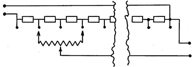
double selector which shunts two of these by a potentiometer having  $2R$  resistance. Of course, the potentiometer could be itself a decimal arrangement of this sort.
