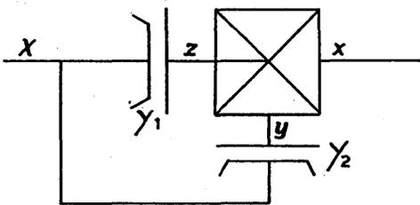
of the differential,  $y$  the negative of the other and  $z$  that of the center wheel. Then
