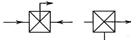
The two side lines indicate the inputs. They may be put in different positions. The output is connected to the middle. The following is a gear box
