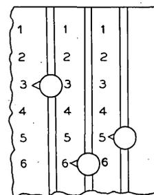
Similarly, we move the pinion in the tens place until it meshes with the rack for the digit 6 and the pinion in the hundreds place until it meshes with the rack for the digit 3. Externally, these operations are performed by moving a knob which projects through a slot. The slot is parallel to the axle of the pinion and the pinion itself is moved by certain projections on the lower and unseen portions of the knob. Thus, we have entered the multiplicand 365.
