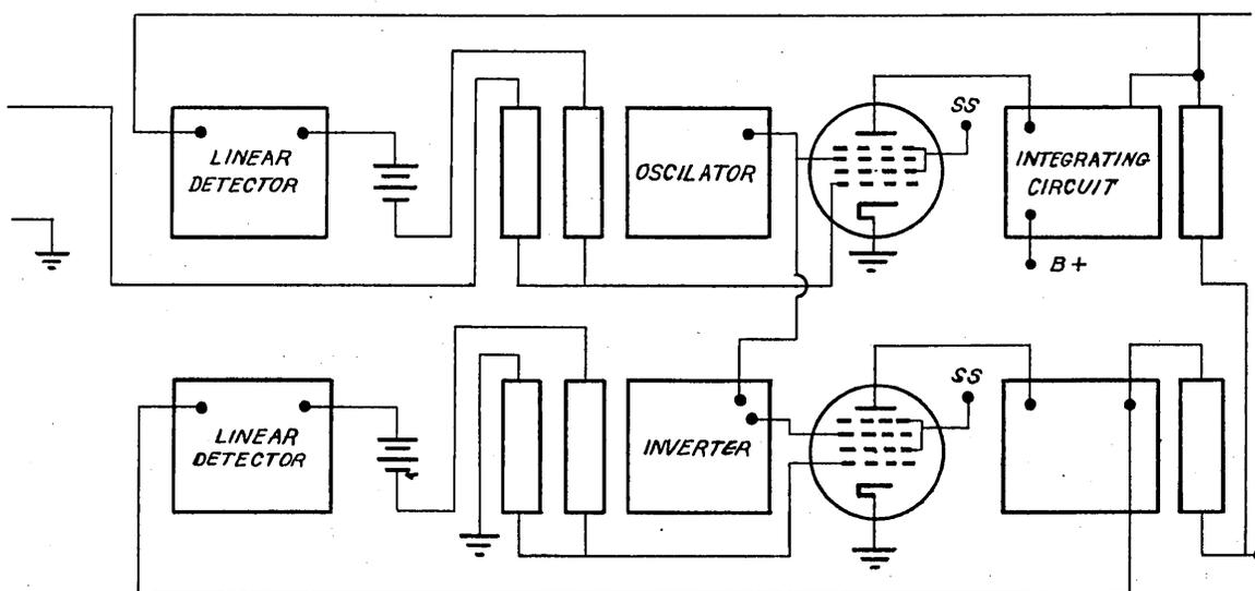
8. For the purpose of electrical multiplication, it is very desirable to have a rectifier whose output is a direct current or voltage which is, to a good approximation, proportional to the square of the amplitude of the impressed alternating current. It is not particularly difficult to compensate to a certain extent for the departure of the output of a diode from a square form. We wish to discuss this question in the present section.
