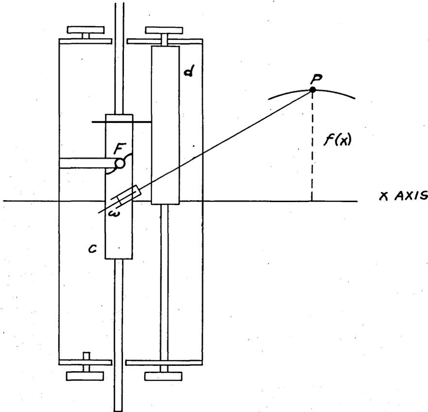
The two integragraph wheels are connected to realize the pair of equations
