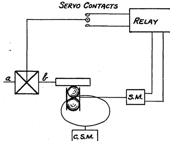
will not work. Here  $a$  is the shaft whose rate of rotation is to be measured,  $b$  is the shaft whose output is to match the other. The output of the differential is the difference of the shafts  $a$  and  $b$ . The servo contact arrangement is such that when  $a-b$  is positive, the servo motor tends to increase  $b$  ( $= \frac{db}{dt}$ ) and conversely when  $a-b$  is negative, the arrangement tends to decrease  $b$ .
