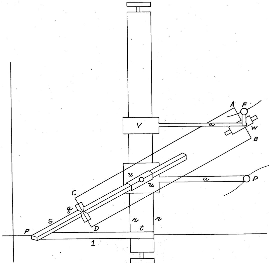
On this carriage we have a pivoted collar through which rides a bar  $s$ . The other end of this bar is pivoted at the point  $p$  which is on a fixed extension of frame. This arrangement of collar and pivot insures that the slope of the bar  $s$  equals  $f(x)$ .
