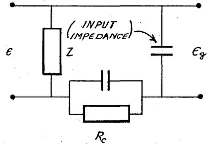
frequencies, the input capacity is negligible but very important in radio and higher frequencies. This also holds for the output capacity which we have entered into  $Z_L'$  in the above.
