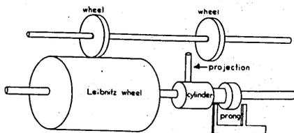
A prong determines the position of this cylinder. Thus when the unit wheel passes from nine to zero, it moves the prong which moves the cylinder on the
