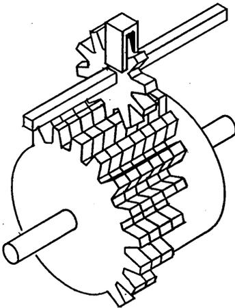
The cylinder and smaller wheel have parallel axis and there is a small pusher, which permits one to displace the smaller wheel along its axle. The axle of the smaller wheel has a square cross-section.
