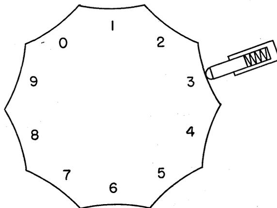
used to insure that the dial comes to rest in one of the ten possible positions. This is very desir-
