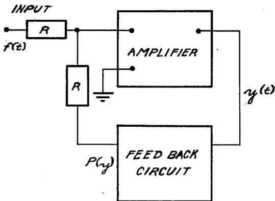
it. The resistances R are equal, consequently the input to the amplifier is the average of  $f(t)$  and  $P(y)$
