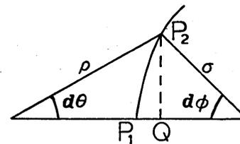
$P_1$  and  $P_2$  are (to the first order) points of contact. The arc length on each C curve is the same  $P_1P_2$  and hence the motion is non-slipping.
