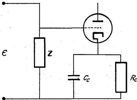
the equivalent of a filter circuit between  $\epsilon$  and  $\epsilon_g$  when one considers that the relationship between the grid and cathode is similar to the plates of a condenser and hence one has a capacitance connection (the "input capacity") between them. For audio
