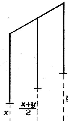
There are a number of ways in which the three rods can be connected so that the specified three points will remain colinear. One may have a cross bar pivoted upon the central bar. This cross bar has a slot on each side in which a pin is fixed on the corresponding rod slides. The pins and the pivot are constrained then to be colinear.
