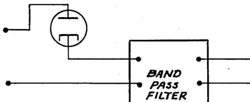
In order to measure accurately the peak voltage of an alternating current, the following circuit is used
