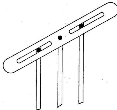
This cross bar arrangement can be replaced by a pantagraph. The bars AC and CF are rigid and equal with midpoints B and E respectively.  $DE = BC$  and  $BD = CE$ .
