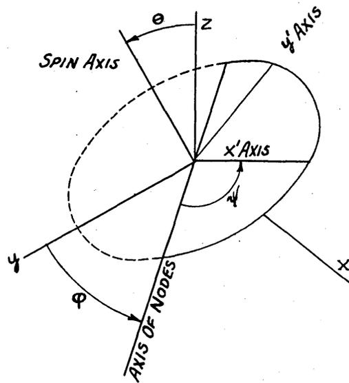
coincides with the spin axis. Consequently the  $x'$  and  $y'$  axes for this body fixed set remain in the plane determined by the axis of nodes and the third axis of our previous discussion.
