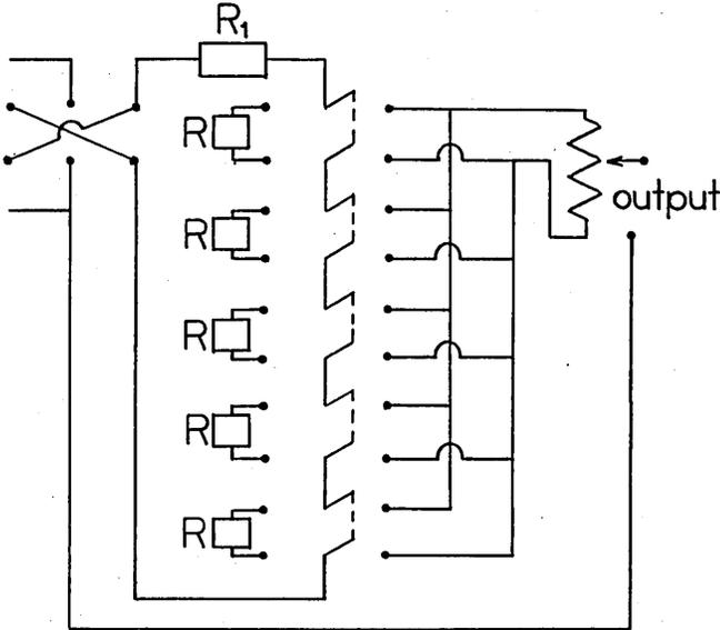
The resistances  $R$  have the value  $P$ , the value of  $R_1$  is  $5P$ . The first d.p.d.t. switch, of course, distinguishes between the  $\lambda$  range, 0 to .5 and .5 to 1.0. Only one of the remaining switches should be thrown to the right. This will insert the potentiometer into the circuit in series with four of the smaller  $R$ 's in same order.
