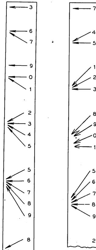
The multiples are obtained as follows: For each digit of the multiplicand, a corresponding strip is chosen and the strips are laid side by side in the order of the digits of the multiplicand. Each multiple is obtained by starting at the right hand of the corresponding row and following the arrows. Due to the slant of the arrows, this procedure accomplishes the equivalent of the addition of pairs of digits of the previous method and also any carrying that might be necessary.
