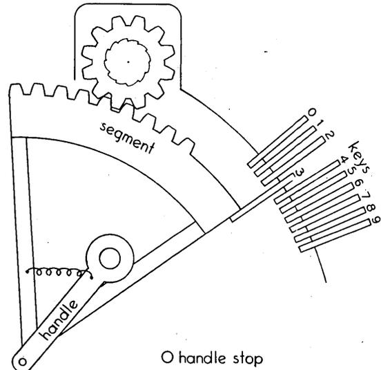
will cause the segment to revolve until it is stopped by whichever one of the ten keys is pressed down. Thus the amount of rotation of the segment is determined by pressing down the key. A portion of the rim of the segment is toothed and gears into a
