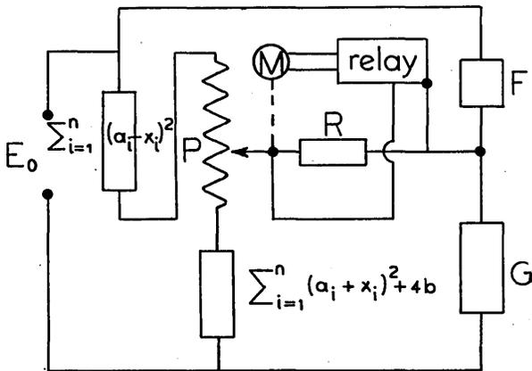
The potentiometer P is linear and if  $y$  corresponds to the displacement of its contact from the midpoint, the resistance of it in one circuit is  $R - 2y$  and in the other  $R + 2y$ . One sees then from our equation that for equality we must have
