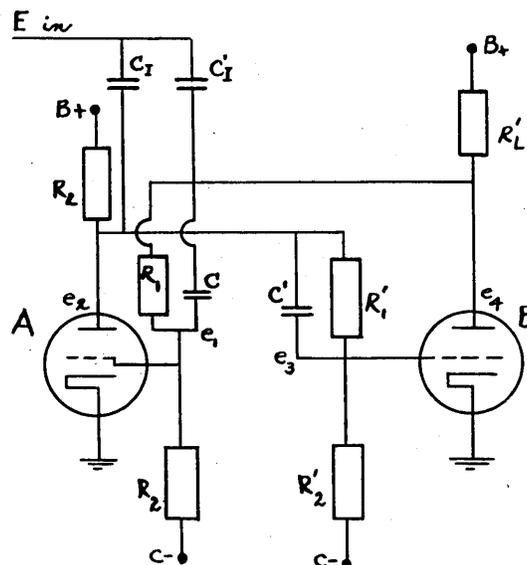
constants are properly chosen. Furthermore a properly shaped input pulse of the correct magnitude will cause this circuit to go from one steady state to the other.
