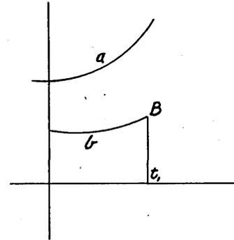
is positive,  $a - b$  is increasing and the servo contacts cause  $\dot{b}$  to increase. Presumably, the motor is effective enough to cause  $\dot{b}$  to overtake  $\dot{a}$  and hence we eventually get to a situation where  $\dot{a} = \dot{b}$ . It is clear that any device which registers the sign of  $\dot{a} - \dot{b}$  can be used instead of the friction coupling indicated.
