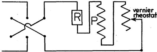
In general, it is not easy to synchronize two potentiometers. However, it is possible to use a second potentiometer to adjust for the variation of total resistance due to the different settings of the potentiometer provided the load is specified. Commercial combinations of this type exist.
