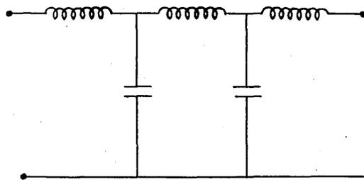
erty that it tends to shunt the non-constant currents but offers little resistance (just that necessarily associated with the inductances) to the direct current.
