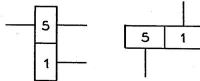
The ratio of rotation of corresponding shafts will be indicated in the boxes by a number, not by the size of the boxes. The possibility of shifting will be indicated as follows:
