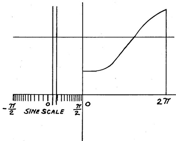
lel to the  $y$ -axis. To set up a rectangle with one pair of sides having the length  $\sin \beta - \sin \alpha$ , we set the wire of one slide on the value  $\alpha$  of the sine scale and the other on the value  $\beta$ . The distance between the wires is then  $\sin \beta - \sin \alpha$ . The  $x$ -axis, the first slide wire and these last two now enclose a rectangle. (This is not the device described by Galle, *loc. cit.*, but the idea is the same.)
