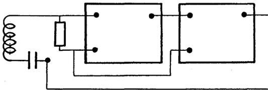
Now if the feedback were adjusted properly, the voltage drop in the circuit which is proportional to the  $i$  would be zero or positive. The resulting current would have an exponential term with a non-negative exponent and hence the current would not die out. The circuit is then said to be oscillating.
