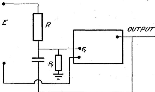
Let  $J$  denote the voltage across the condenser. Let  $R_i$  denote the resistance between the input and the ground in the amplifier (sometimes this may be neglected). The current  $i$  through the resistance  $R$  is easily seen to be
