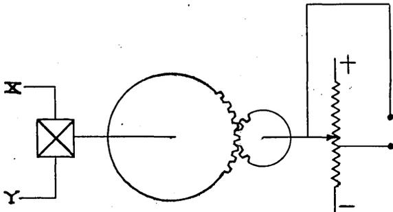
If the potentiometer is connected to  $X - Y$  by a gear arrangement with a partly toothed gear on the  $X - Y$  shaft, then the motion of the  $X - Y$  shaft is not restricted as much as by the previous arrangements. However, if a straight potentiometer connection is used one has a voltage proportional to the difference.
