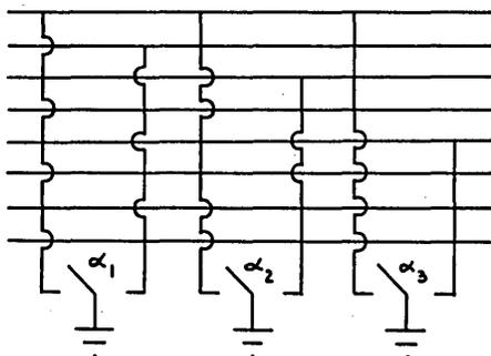
Notice that for each choice of positions for all the switches one and only one channel remains ungrounded. If the signals are all of given polarity, only one diode is necessary for grounding. A matrix selecting switch system can also be used in multipliers to obtain the two digits in the split multiplication table method and circuits of this type were originally developed by Rajchman and Crawford for this purpose. Multiple contact relays are used for selection also.
