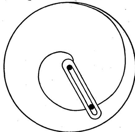
x pivot along the y bar, according to the amount of relative motion between cam and bar. Hence, if the bar is turned an amount y, we must turn the cam an amount y + x. This can be accomplished by means of a differential which adds the two inputs x and y. In the screw case the situation is similar.
