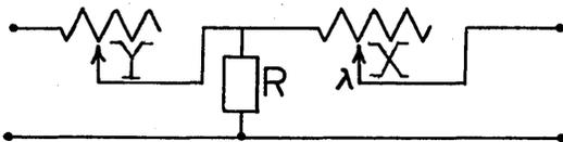
Here x and y are variable resistors connected so that  $x = R/\lambda - 2R$  and  $y = R\lambda$ . It is readily seen that for every value of  $\lambda < \frac{1}{2}$ , the total resist-
