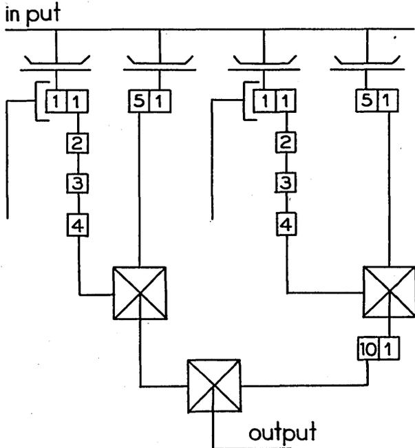
(There is little practical difficulty in arranging the indicated gear shift.) Notice that the output can be any multiple from 0 to 99 of the input.)
