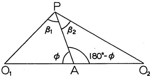
The lamina  $D_2$  will rotate an amount  $\theta_2$ . At P, the normal component of the motion must be the same for each lamina if they are to remain in contact. (In general, the laminas will slip relative to each other, but this corresponds to a difference in the tangential components of the motion of the laminas at P.) Thus,  $\theta_2$  is determined approximately by the equation
