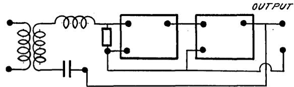
Such a circuit can be used as a selective alternating current integrator. Theoretically it is the precise generalization of the direct current integrator of the previous section based on a condenser. Let us consider what happens when  $n$  cycles of a voltage  $\alpha \sin \omega_1 t$  is impressed on such a circuit. We suppose that the turns ratio of the transformer is one. Thus we have a voltage  $\alpha_1 \sin \omega_1 t$  impressed on a circuit which is essentially
