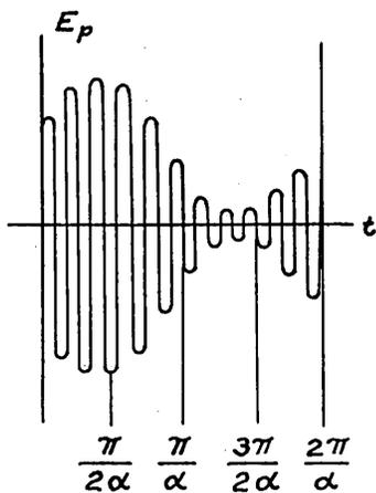
If the voltage  $E = (A \sin \alpha t + 1) \sin \omega t$  is applied to the plate of a diode we obtain a current
