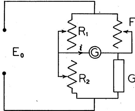
Since  $F$  and  $R_2$  are linear rheostats, the inputs can be considered as a rotation. The output can also be obtained as a rotation if  $R_1$  is a linear rheostat turned by a "servo motor."
