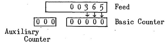
counter. The auxiliary counter has a unit feed in the units place. Since we have added twice, this extra feed has been applied twice to the units place of the auxiliary counter and hence it reads 2. We now shift the feeding mechanism relative to the counters.
