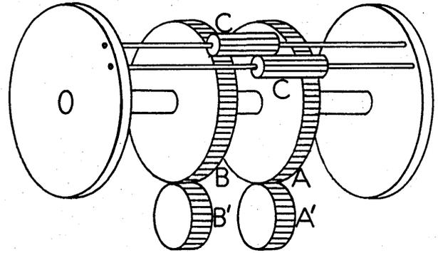
Thus if the inputs  $x$  and  $y$  are applied to A and B, and  $z$  is the rotation of the C gear mounting, then the relative motion of A to C, i.e.,  $x - z$  must equal the relative motion of C to B, i.e.,  $z - y$ . Hence,  $x - z = z - y$  or  $x + y = 2z$ .
