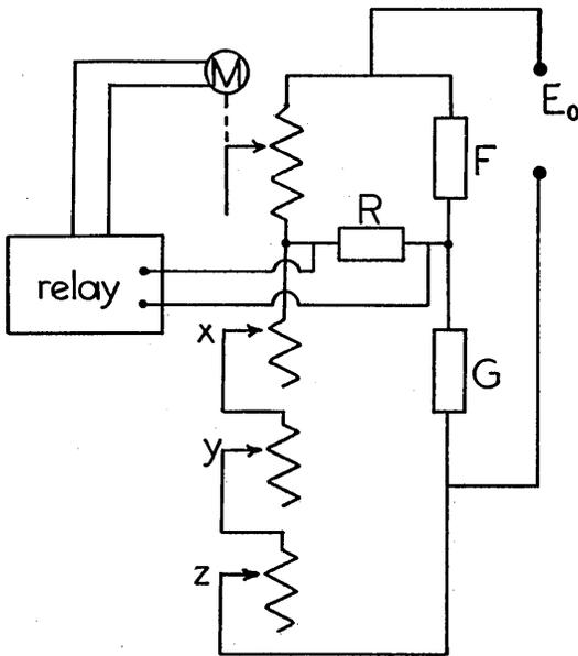
If  $R_0$  is the value chosen as unit resistance, the maximum resistance for  $x$  should be  $3R_0$ , that for  $y$  and  $z$   $2R_0$  and for  $w$ ,  $7R_0$ . This illustrates the convenience of logarithms when one has to deal with greatly varying quantities. However, this has its difficulties too as we shall see.
