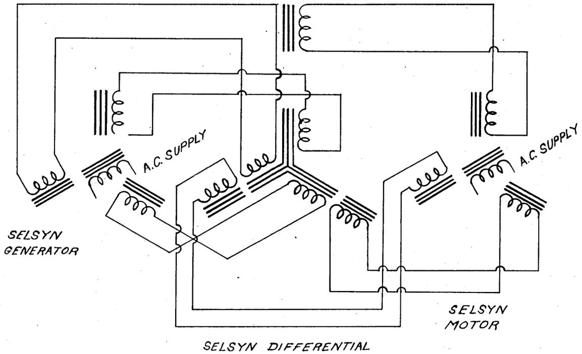
calculating devices because it permits one great freedom in connecting various units. Thus in the latest version of the differential analyzer at M.I.T. a selsyn system (based on capacity, however,
