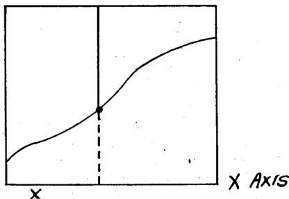
a piece of paper on a vertical drawing board. As we mentioned above, in this case we have a continuous input  $x$  and the drawing board is continuously displaced to the left with this input. Thus while the pencil remains in the same vertical plane, the graph of  $y$  appears on the drawing board.
