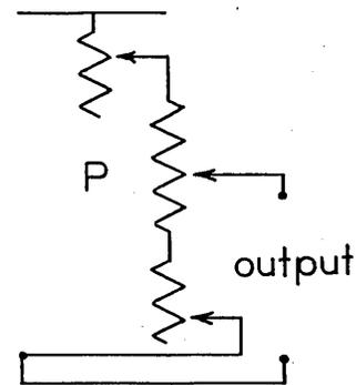
Let  $P$  denote resistance of the potentiometer. Now if we have added  $\delta_1 P$  from the lower rheostat and  $\delta_2 P$  from the upper rheostat, we have the equivalent of replacing the potentiometer  $P$  with setting  $\lambda_0$ , by a larger potentiometer, in which the total
