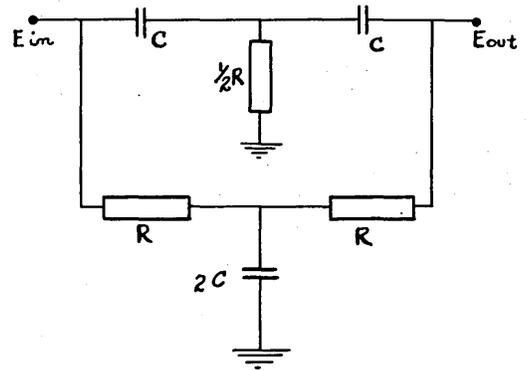
The discriminated frequency is again given by  $f_0 = 1/2\pi RC$ . The nodal equations readily yield for any frequency  $f$ , if  $\rho = f/f_0$ , that  $E_{out} = E_{in} i(\rho - \frac{1}{\rho})/[4 + 2R/R_L + i(\rho - \frac{1}{\rho}[(1 + 2R/R_L)])]$  if  $R_L$  is the resistance connected across  $E_{out}$ .
