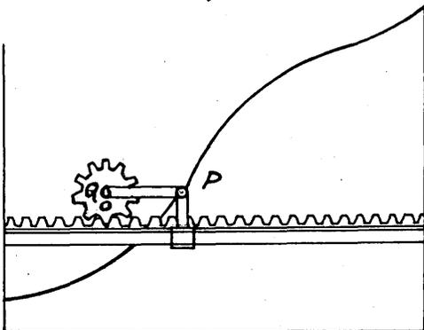
line of the rack has an ordinate which differs from that of P by a fixed amount. Another connection to the pinion insures that the center of the wheel has the same ordinate as P and the abscissae differ by a constant. The rate of rotation of the pinion is determined by the choice of the radius. There is a hole in the pinion in which the follower of a planimeter is inserted to trace the Q curve.
