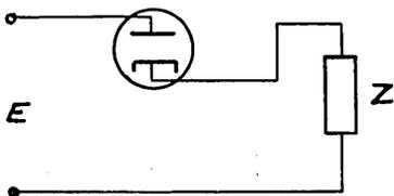
But probably graphical methods offer the most direct method of attack on the problem of studying the actions of vacuum tubes. Thus in the most common form of the problem of detection, we have an impressed voltage in the form  $E = (A \sin \alpha t + 1) \sin \omega t$  where  $\omega$  is much larger than  $\alpha$ . The problem is to obtain a voltage proportional to  $A \sin \alpha t$ .  $\nu = \omega/2\pi$  is the carrier frequency,  $A \sin \alpha t$  is the modulation.
