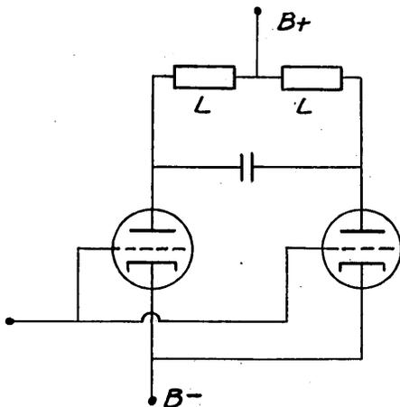
If the tube A is conducting and B is not, there will be a considerable voltage drop across the condenser. If now the grids are excited, tube B will become conducting. This lowers the voltage on the B end of the condenser and, of course, the A end is also lowered. If the voltage fall of the A plate is adequate, the A tube will be quenched.
