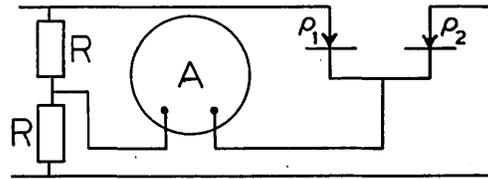
clear that if the voltage across the rectifier  $\rho_1$  is  $e_1$ , that across the rectifier  $\rho_2$  is  $-e_1$ . (We neglect the current drawn by the rectifiers here.) Consequently the current through  $\rho_1$  is
