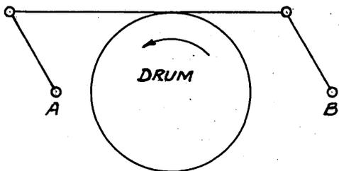
a band, which passes once around the drum and then to B. If now we pull on A, then the band tightens on the drum and the lever B is pulled by a force which is augmented by the pull of friction between the band and the drum.
