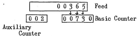
We next apply the feed mechanism three times. This adds 10950 to the basic counter and changes the auxiliary counter by three in the tens place. We again shift the feeding mechanism.
