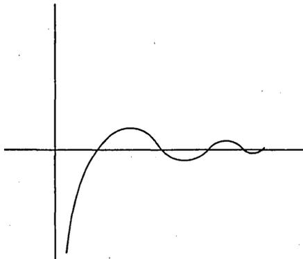
After the first maximum, the curve can be compared essentially with  $e^{-\alpha t} \sin \omega t$ . If the ratio of successive maxima is fairly constant this can be considered as a measure of damping. If the times between zeros are relatively constant they can be termed half periods.
