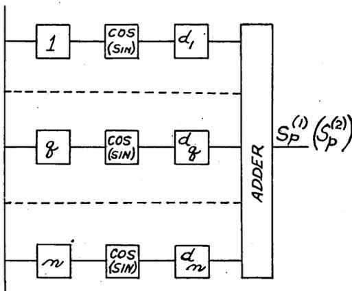
This arrangement is such that if we replace the input  $p \pi/n$  by a continuous variable  $x$ , we get the sums
