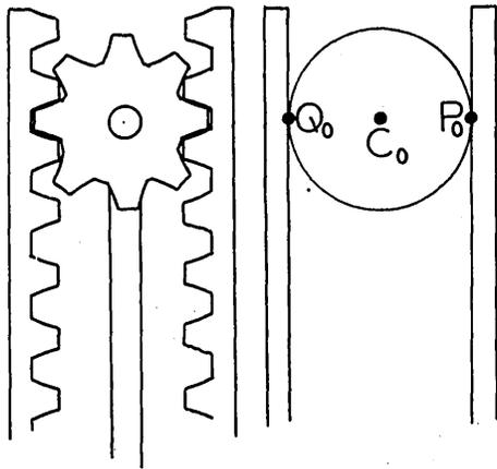
for the center of the wheel and its points of contact to the two bars. Let  $C_1, P_1, Q_1$  refer to the corresponding points fixed on the circle  $P_2, Q_2$  the corresponding points fixed on the bars. Now if the system is moved to a new position in which P and Q are the new points of contact, we see that since the wheel did not slip relative to the bars that  $P_2P = P_1P = Q_1Q = Q_2Q$ . Since  $C_1P = C_1Q$ , this yields that  $P_2, C_1$  and  $Q_2$  are colinear.
