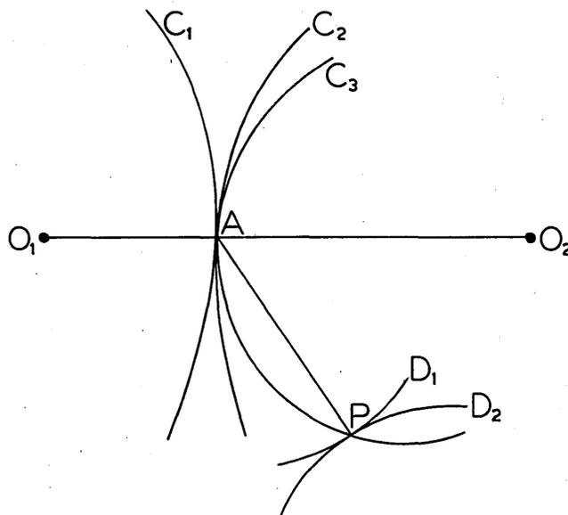
The point P is common to the curves  $D_1$  and  $D_2$ , since this is a position corresponding to contact of  $C_3$  with  $C_1$  and  $C_2$  at A. Since  $C_3$  is rolling on the other curves in each case  $D_1$  and  $D_2$  have a common normal AP at P from the above. Thus,  $D_1$  and  $D_2$
