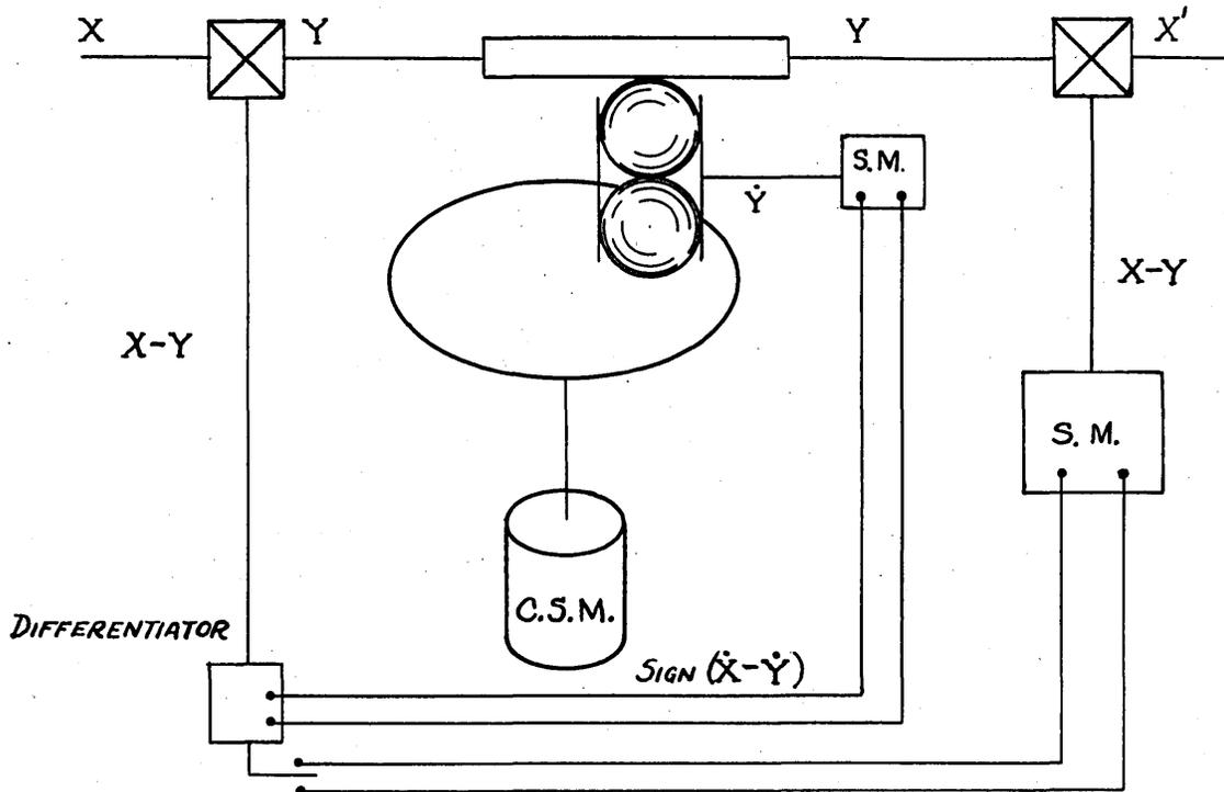
amounts of light enter both phototubes. A variation from this position by the output shaft will favor one or the other phototube and hence can be used to control a servo. (Cf. Berry, T. M., *Trans. Amer. Inst. Electrical Eng.*, LXIII (1944), p. 195).
