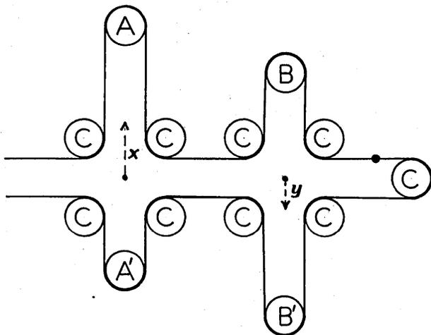
wheels are fixed in position, the wheels A, A' are a fixed distance apart and similarly the pair B, B'. If we move the pair A A' along their line of centers an amount  $x$  and the pair B B' an amount  $y$ , then a point R on the chain will move an amount  $2(x+y)$ . It is clear that this can be applied to any number of addends. In the drawing,  $y$  is negative.
