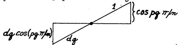
The method of addition that is used is very interesting since it is a mechanical counterpart to the voltage averaging which we have previously discussed. Let us describe it in the case of two addends since this case contains the essential ideas. Suppose we have a cylinder which can rotate
