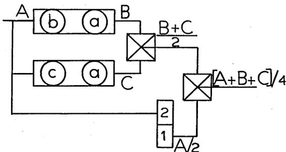
In this device, we continue to feed in A, starting (say) with  $A = 0$ . The outputs of the two links multipliers will be the acute angles B and
