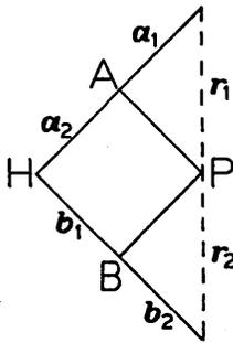
If the desired ratio is  $r_1/r_2$ , we must first choose A so that  $a_1/a_2 = r_1/r_2$  and B, so that  $b_1/b_2 = r_1/r_2$ . We then must fix the lengths of the remaining arms so that  $AP = b_1$  and  $BP = a_2$ .
