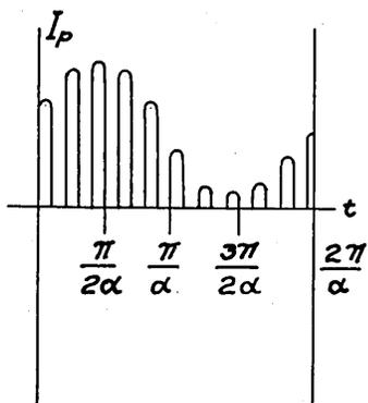
For  $I_p$  we have a constant component  $i_0$  obtained by averaging. We also have a component  $i_\alpha \sin \alpha t$ , since it is clear that  $\int_0^{2\pi/\alpha} I_p \sin \alpha t dt$  is not zero. (Notice that  $I_p$  is largest when  $\sin \alpha t$  is
