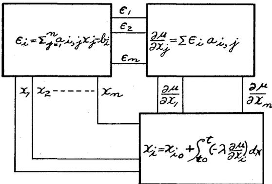
Notice that we have established the stability of this device. An arbitrary feedback, for instance,  $\frac{dx_i}{dt} = \lambda \epsilon_i = \lambda (\sum_{j=1}^n a_{i,j} x_j)$  is not stable except for special matrices  $[a_{i,j}]$  as one can readily see by solving this system of differential equations.
