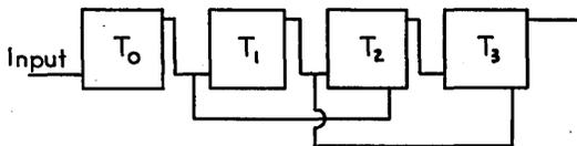
to (1,1,0,0) in response to the first three pulses. As above the effect of the next pulse is to send it to the (0,1,1,0) stage, i.e., the counter passes from 3 to 6 skipping two states. The next state is (1,1,1,0) or 7. The next pulse, at first, clears the system to (0,0,0,1). However, there is also a feedback from the last stage so the circuit goes to (0,0,1,1) or 12. [One would also expect that when  $T_2$  turns to 1 from 0 in this process,
