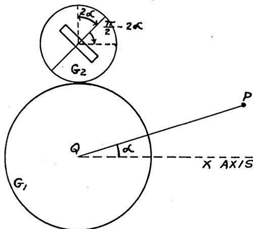
Mounted on  $G_2$  there is an integrating wheel, whose point of contact with the paper is on the axis for  $G_2$ . The integrating wheel is arranged so that when  $\alpha = 0$ , its angle is perpendicular to the x-axis. Consequently when PQ rotates through an angle  $\alpha$ , the axle will turn through an angle  $2\alpha$  and make angle  $\frac{\pi}{2} - 2\alpha$  with the x-axis.
