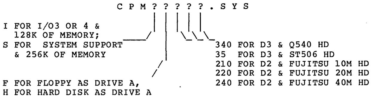
For example, a file named CPMSH340.SYS supports the SYSTEM SUPPORT serial port as its system console port, 256 Kbytes of memory, and a DISK3 with a Quantum Q540 hard disk.
