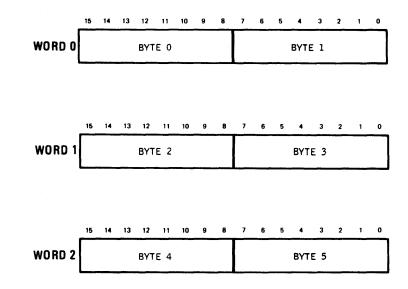
Figure 1-4. Data in Memory, Two Bytes Per Word
