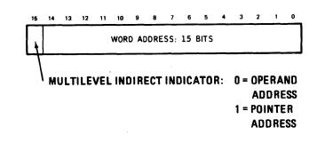
Figure 1-7. Indirect Address Pointer Format
