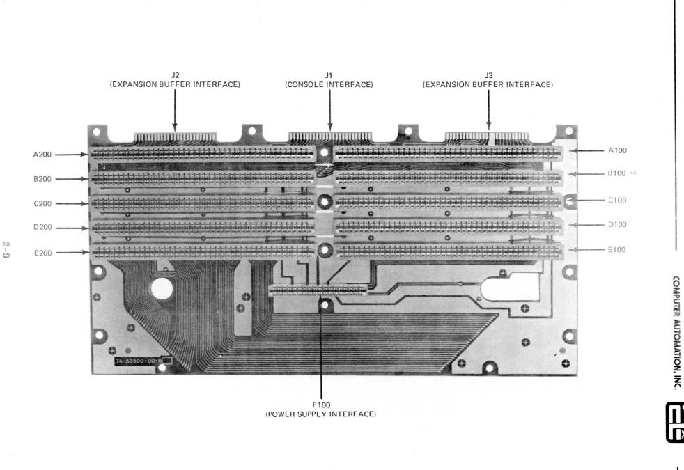
Figure 2-2. ALPHA LSI Motherboard Slot Organization (Rear View)
