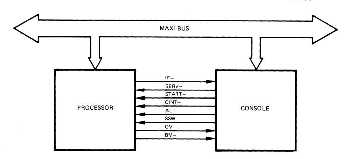
Figure 9-1. Processor/Console Interface
