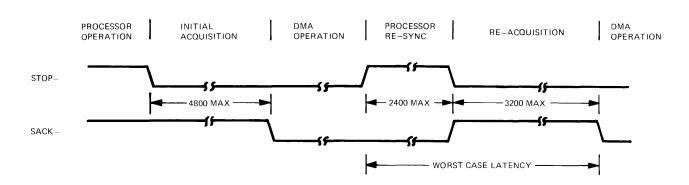
Figure 6-1. Maxi-Bus Acquisition Timing
