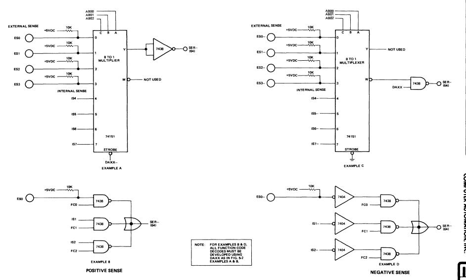
Figure 5-5. Positive and Negative Sense, Circuit Configurations
