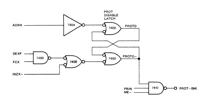
Figure 5-9. Reentrant Interrupt Implementation
