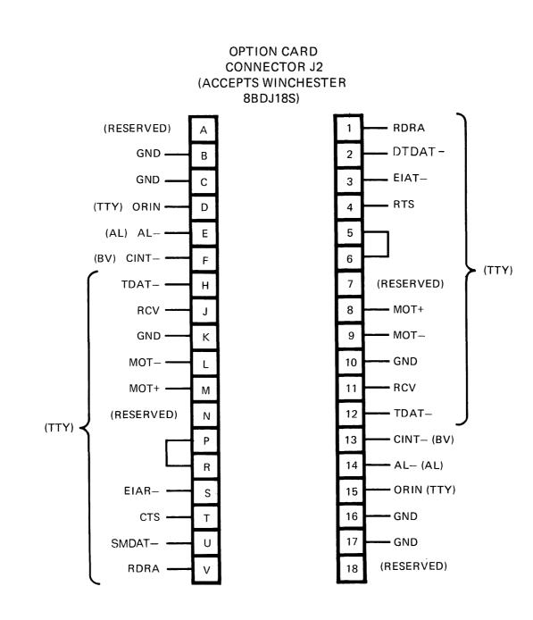
Figure 11-2. Option Card Connector J2 Pin Assignments
