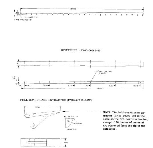
Figure 7-3. Standard Circuit Board Hardware
