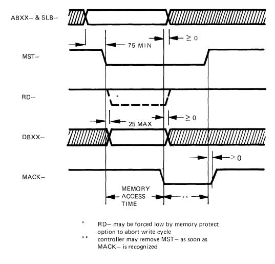
Figure 6-4. Write Access Timing
