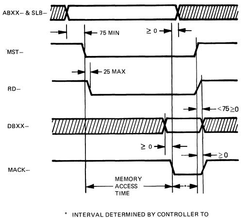
INTERVAL DETERMINED BY CONTROLLER TO ACCEPT MEMORY DATA
