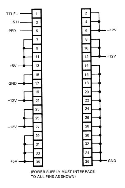
Figure 10-4. Motherboard Power Adapter Pin Assignments.
