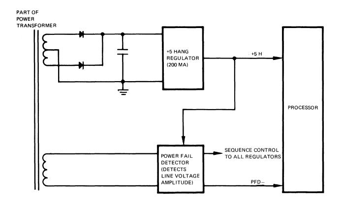
Figure 10-1. Power Monitor Block Diagram.
