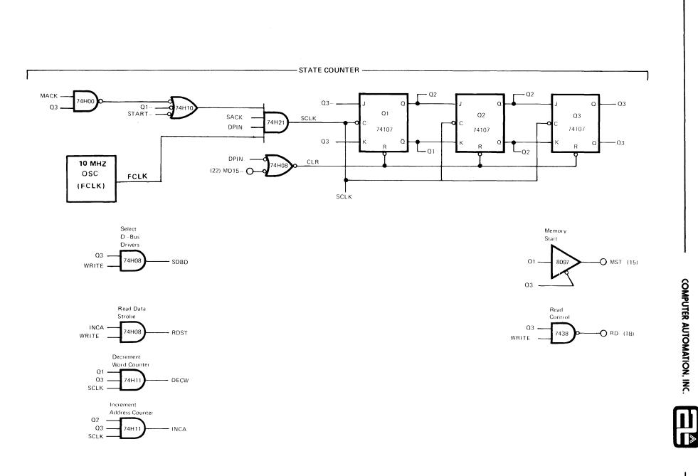
Figure 6-7. State Counter and Decoder
