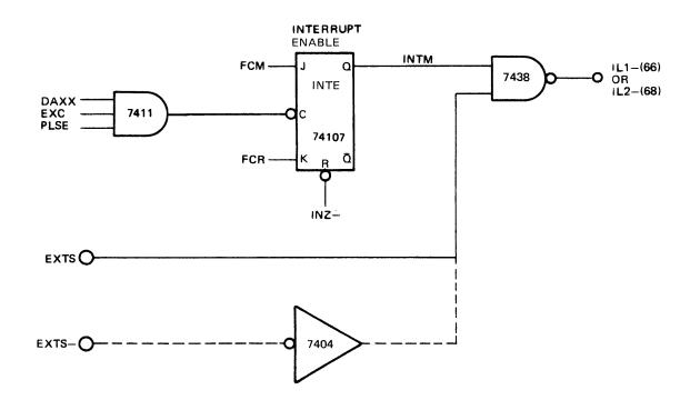
Figure 5-10. Simple IL1-/IL2- Interrupt Structure
