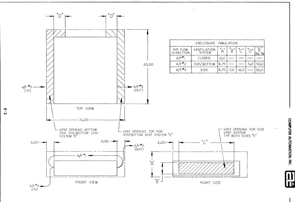
Figure 8-2 ALPHA LSI Ventilation Systems
