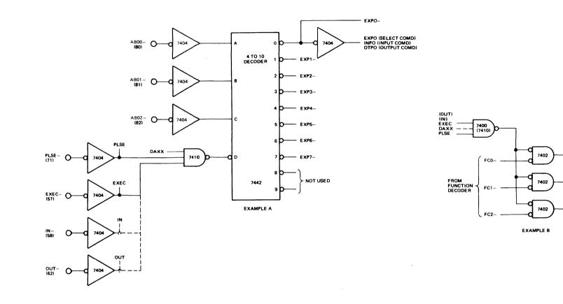
Figure 5-3. Select, Input or Output Command Decode Configurations
